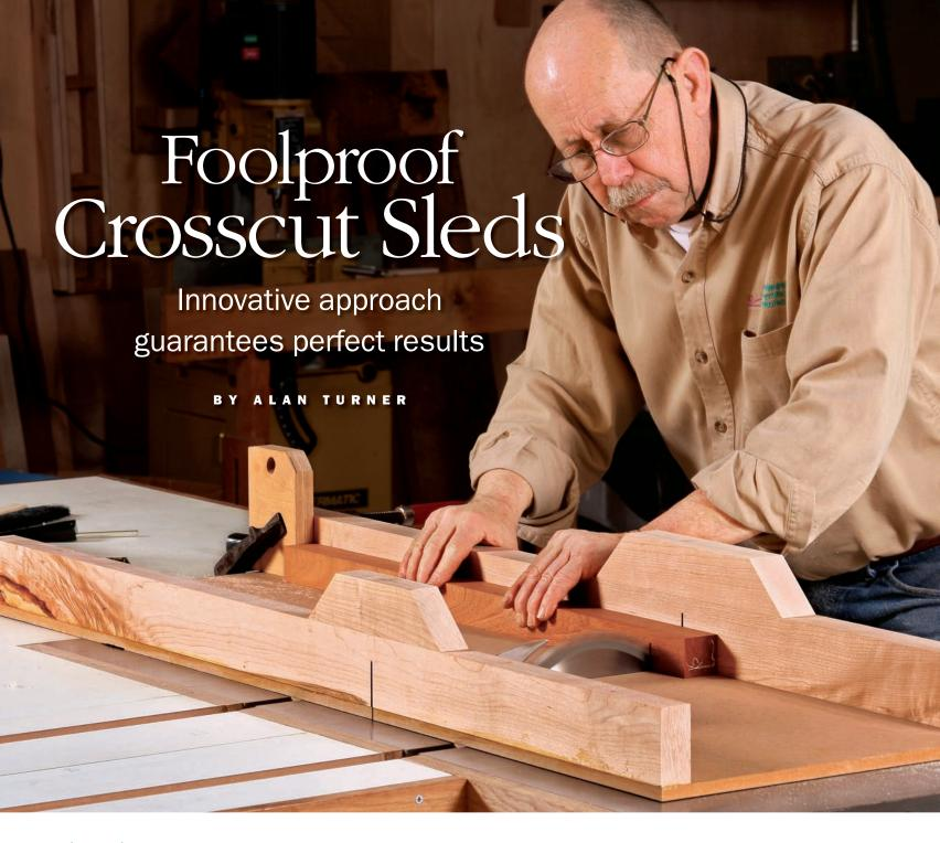
he tablesaw may be your shop's most valuable cutting tool, but for precise, repeatable crosscuts it needs a little help from a sled. The sled holds the work securely with its long edge at a precise right angle to the blade, so you get perfectly square ends when cutting pieces to length, the key to gap-free joinery. With a zero-clearance slot cut through it, the sled even prevents chipout at the edges.
