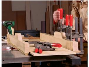
Put the glue-up in clamps. Then, after the glue dries, drive a series of screws from underneath to complete the assembly.
