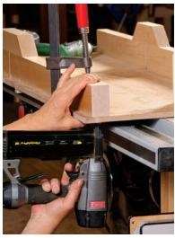
**Nail the other end.** The nail will flex just enough to allow subtle adjustments to the fence's position, but will otherwise hold the fence in place.
