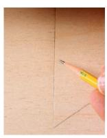
**Butt the pieces together.** A gap indicates that the fence is slightly out of square.
