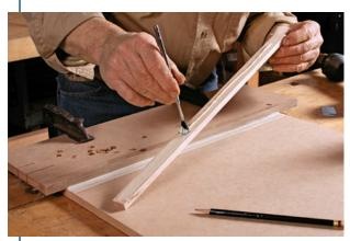
**Glue the runner in place.** Turner uses an MDF template clamped to the sled's base (above) to help locate the runner and ensure it is straight. While pulling the runner against the MDF template, Turner secures it with 18-gauge nails (right).
