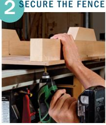
**Apply glue and one screw.** The fence will pivot on this screw while you adjust it to its final position.
