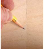
A tap closes the gap. First mark the base with a pencil line to help show the fence's movement. A new test cut shows no space between the workpiece and offcut (right).
