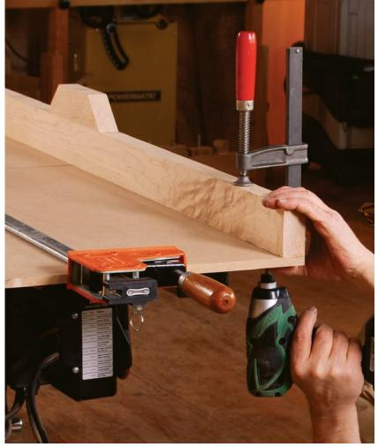
**Screws hold the fence.** With the front fence glued down, Turner drives a series of screws into pre-drilled holes to lock it in place. Its squareness is not critical.
