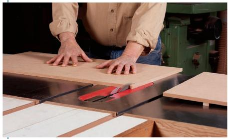
**Trim each base for a perfect fit.** With the runner in the miter slot, cut away the excess MDF. The resulting edge is a perfect zero-clearance fit against the saw's blade.
