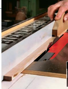
Mill the runners. Start by cutting the pieces oversize to relieve internal stresses that might cause the wood to move. Then trim them to final dimension. Orient the grain as shown so that most of the swelling or shrinking will be vertical and will not affect the runner's fit in the slot.
