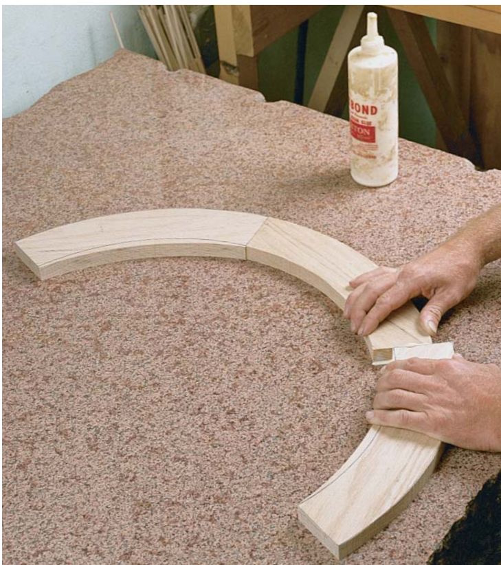
Gluing up the segments. To form rings, apply glue to the ends of the segments; then rub the ends together to force out any air from the joints. A polished stone slab, as flat as a patternmaker's surface plate, makes an easy-to-clean assembly table.
