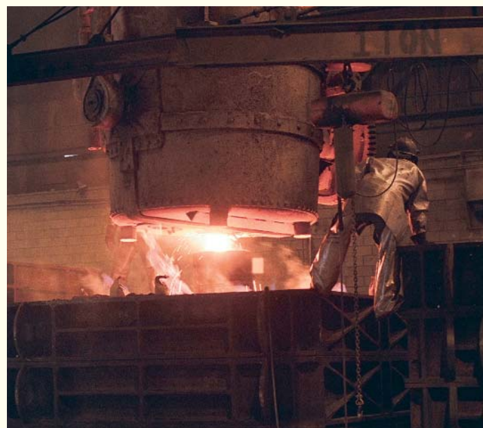
Guiding molten metal at the foundry —Wearing a fire-proof suit, a worker at this Atchison, Kan., foundry guides a ladle as it pours liquid-hot alloy. The flask (frame), containing compacted sand, has an upper (cope) mold and a lower (drag) mold that were formed with wooden patterns.
