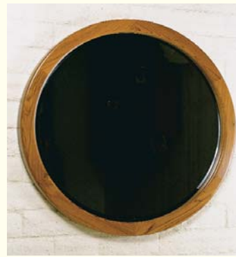
It's hard to tell this mirror frame is made of segments. The reason is that all the joints between segments and between layers are tight.
