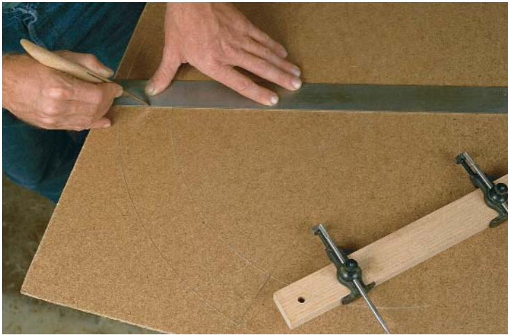
Tempered hardboard is ideal for templates. Use a trammel, a straightedge and a knife to scribe a template for a segment of a circular frame. Then trace the template onto stock.
