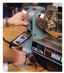
You need to **change speed** based on the project size and material. To do that on most lathes, change the orientation of the belt drive.
