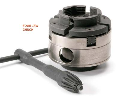
Chucks grab onto a turned piece, most commonly bowls and vessels, and allow the face to be turned without the tailstock intruding. A four-jaw chuck grips a tenon or mortise that is carved by the turner or otherwise attached to the workpiece. Its scrolling action allows it to grab a range of stock sizes and shapes, making it a convenient way to hold work whether between centers or off the headstock only.
