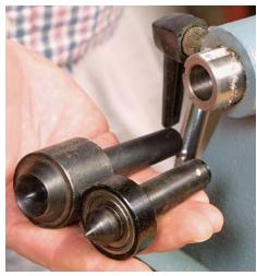
Mounted in the quill, **live centers** spin with the workpiece and apply pressure via a hand screw against the drive center. A live center rotates on bearings with the workpiece while a dead center remains stationary.
