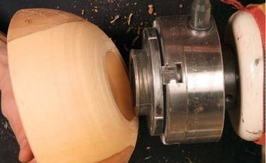
Much like a faceplate (below), **four-jaw chucks** are an alternative holding method. They grab the bowl or vessel with clamping jaws, either grabbing onto a turned tenon (top) or expanding into a turned mortise (above).
