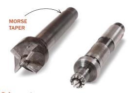
**Drive centers** mount on the spindle and drive the work through a center point and gripping spurs.
