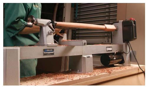
A term integral to making spindles, **turning between centers** refers to turning an item captured between a drive center on the headstock and the live or dead center on the tailstock.
