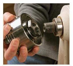
The **spindle** transfers power. It is the driven portion of the lathe and can accept all manner of accessories, like a chuck (shown) or drive center, via its threaded shaft or Morse taper.
