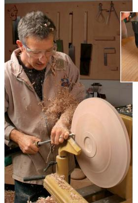
Bowls and vessels also can be turned using a **faceplate**, which screws to the face of a blank and mounts to the headstock spindle.
