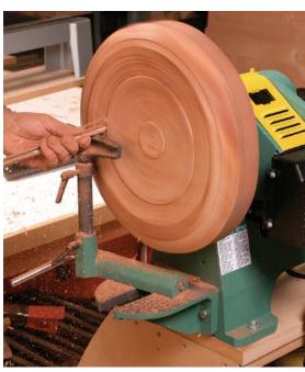
Some lathes allow **outboard turning** of oversize bowls and vessels on the other side of the headstock, where the bed won't interfere.
