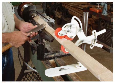
**Steady rest.** Especially in long spindle work, a steady rest can be used to help dampen any vibrations.
