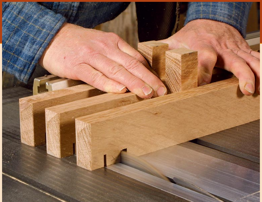
Notch the gridwork on the tablesaw. Insert filler blocks between the long parts of the grid to keep them from flexing during the process.
