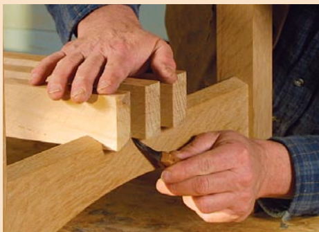
Mark the gridwork for its lap joints. After lightly planing the whole assembly, set it in the stretcher notches and scribe its mating half-lap joints.
