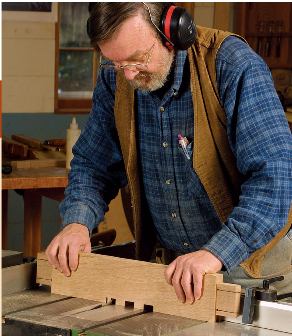
Before assembly, notch the stretchers. Use the tablesaw to notch the arched stretchers for the gridwork. For uniform results use the same fence and stop setup for the two outside notches.
