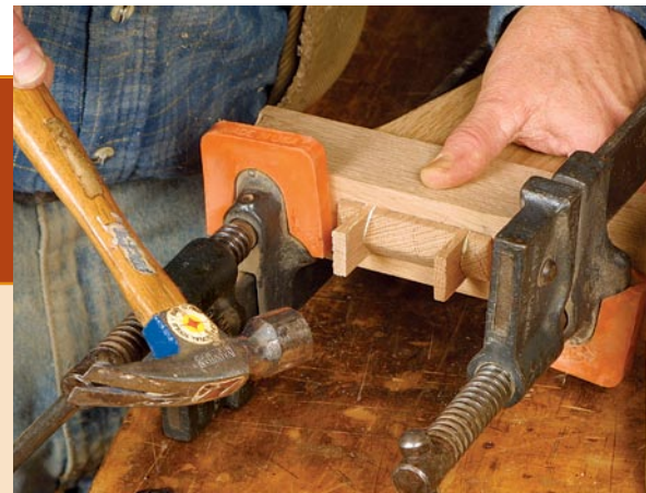
Drive and trim the wedges. During glue-up, drive in the two wedges evenly (top) to ensure proper assembly. After the glue has set, use a chisel to trim the wedges flush with the beveled ends (bottom). Use sandpaper to clean up the surface, including any glue residue.
