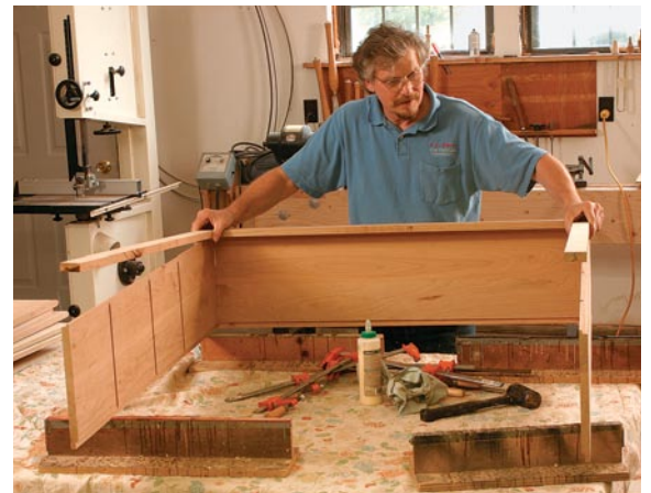
Add the front face frame. For a good fit, rip the rail and stiles so that they're a hair proud of the case, then plane the frame flush to the sides after the glue dries.
