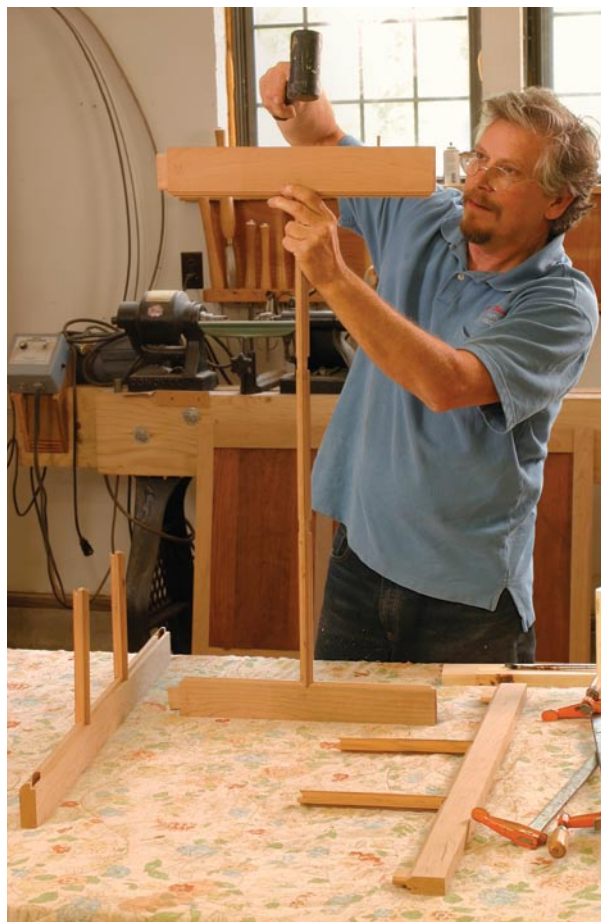
Assemble the door frame. Drive the horizontal muntins into the stile mortises, then install the vertical muntins in the rails (above). Elevate the frame so you can get clamps underneath, then bring all the parts together (right).
