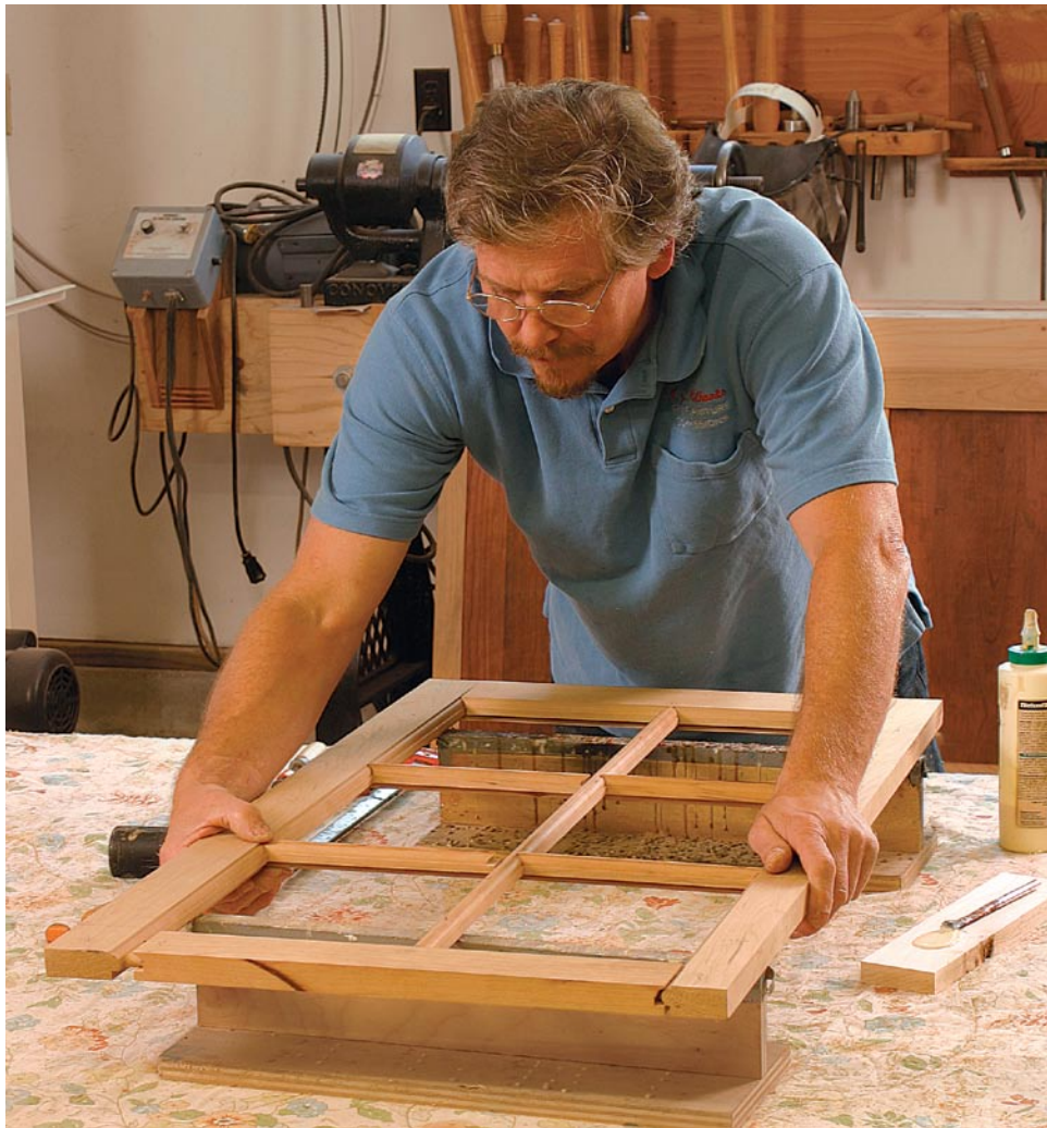
Assemble the door frame. Drive the horizontal muntins into the stile mortises, then install the vertical muntins in the rails (above). Elevate the frame so you can get clamps underneath, then bring all the parts together (right).
