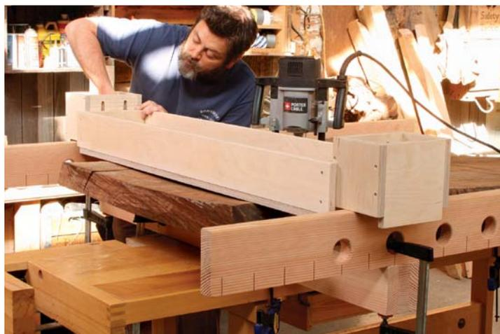
**Adjust the height of the jig.** The extension wings allow up-and-down adjustment, with guidelines on the ends to help you keep the jig level. Adjust the trough so it just clears the highest point of the slab.
