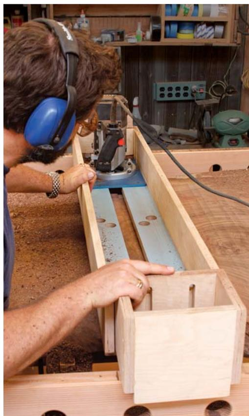
**Lining up a pass.** Just slide the jig over, looking through the bit slot to see the edge of the last cut. You don't need to clamp the jig to the rails.
