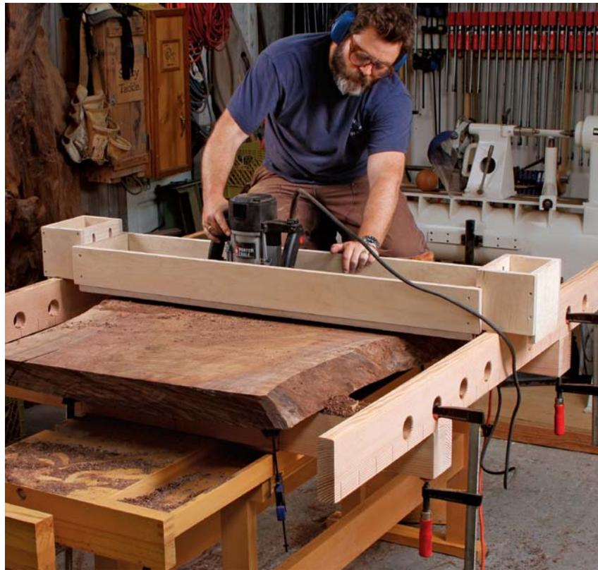
**Hit the high points first.** Just slide the router along the trough to make a pass. One hand is enough to control it unless you hit a knot or other rough patch. Don't force the action. Make the final pass only about  $\frac{1}{16}$  in. deep for cleanest results.
