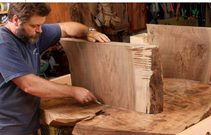
**Place and trace the feet.** Offerman leveled a smaller slab to make these feet. He decides where they will go on the underside of the tabletop, and then traces their location.
