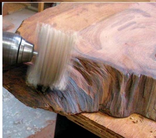
**Don't forget the edges.** Offerman uses a variety of tools, such as this "sanding star" drill attachment (\$18 at woodcraft.com), to remove debris from the edges and prep them for finishing.
