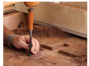
**Room for joinery.** Offerman uses a trim router to carve out extra landing pads for the buttons he uses to join the feet to the slab, squaring them up by hand with a chisel and mallet.
