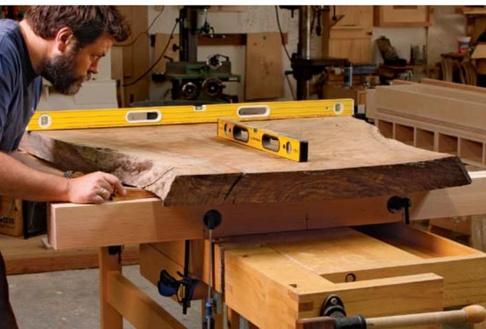
**Level the slab.** After leveling your workbench or worktable, clamp the support beams to it. Then the slab goes on and gets leveled. The idea is to even out the high or low points as much as possible to maximize the finished thickness. One long and one short level, plus a few shims, are all you need. Big workpieces like this will stay in place without clamps.
