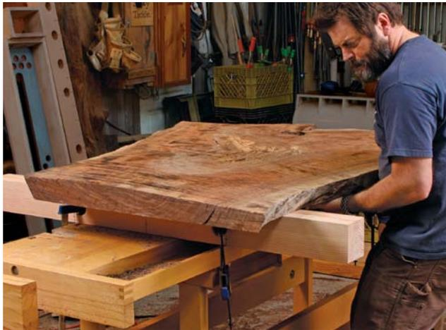
**Grip it and flip it.** Tip the slab up on edge, and balance it there while you sweep the shims and dust off the rails. You might need some help. Then lay it down flat on its other side. Take a moment to enjoy how it lies perfectly flat on the support beams.
