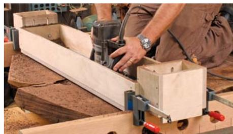
**Lock the jig in place.** A few clamps on the rails are necessary to keep the jig from sliding sideways, and a few passes get you to finished depth. Then move the jig over, lock it in place, cut to the same depth, and repeat until you've created a trough wide enough to accept the foot.
