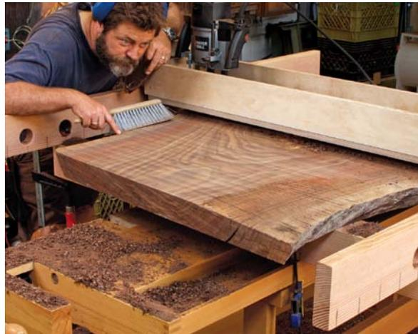
**Route the other side.** You'll be surprised at how quickly the whole process goes, leaving smooth rows of router tracks on both sides of the slab.
