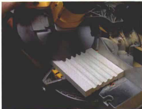
Vertical is better. Although a compound-miter saw can cut a wider bevel with the board flat on the table, a vertical cut—with the board held upright against the fence—is faster, easier and more accurate.
