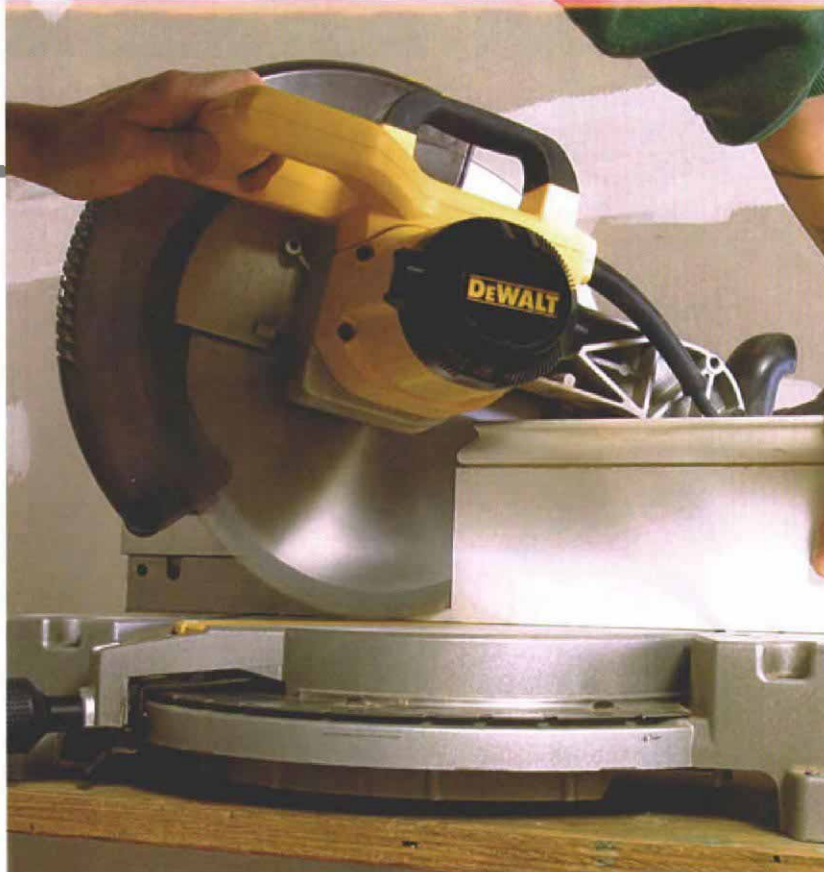
Vertical is better. Although a compound-miter saw can cut a wider bevel with the board flat on the table, a vertical cut—with the board held upright against the fence—is faster, easier and more accurate.
