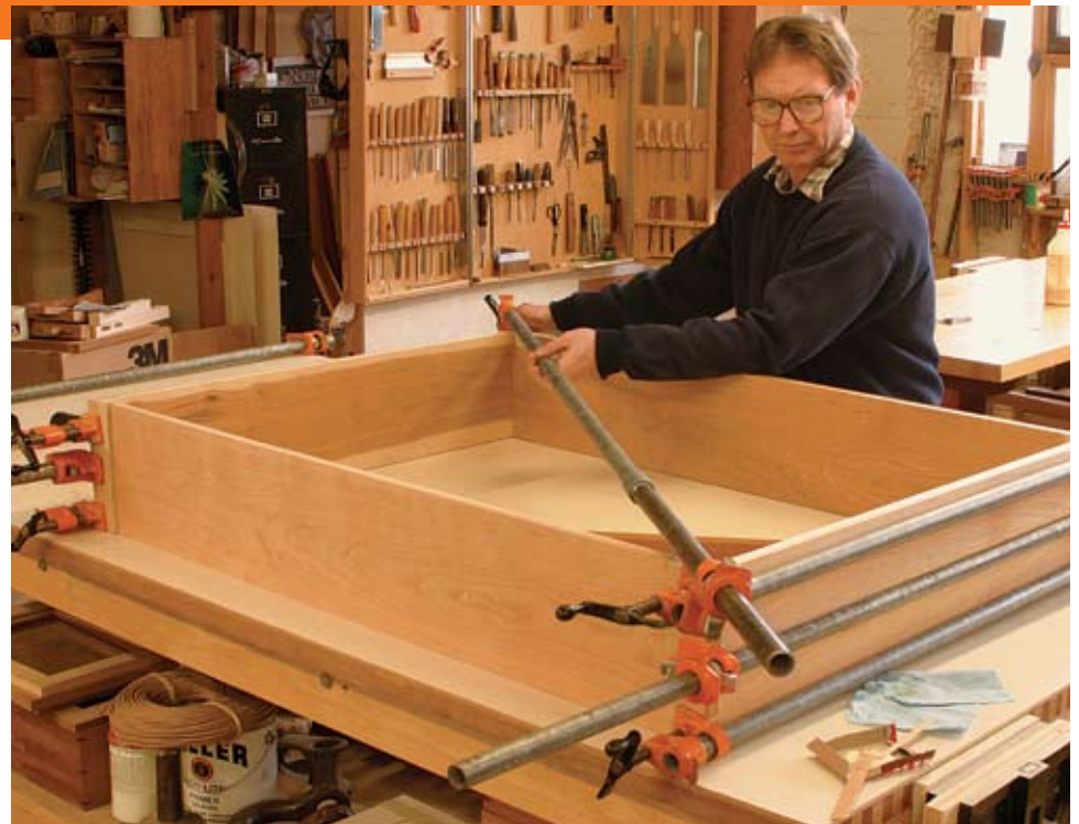
Use melamine cauls and check the diagonals. On dovetails, Rogowski keeps the long grain proud, which allows him to use flat cauls. Later, he planes the sides flush with the pins and tails. If the diagonals don't match, use a long clamp to draw the assembly square.
