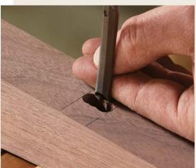
Drill for attaching the tabletop. The screw holes and counterbores in the shorter arm need to be slotted to allow for wood movement in the top. Do that by overlapping holes and clearing the waste between them with a chisel.
