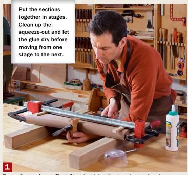
**Two column pieces first.** Start by gluing the two short-axis column pieces together, using a spline to align them. Use a long bar clamp to ensure that the ends of the tenons and their shoulders end up dead even.
