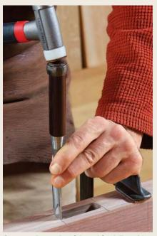
**Square the ends with a chisel.** To guide the chisel, knife a line at each end of each mortise.
