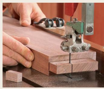
**Trim on the bandsaw.** Hold the column parts against the arms and feet to mark where to trim each tenon. Make the shoulder cuts at the tablesaw and then use the bandsaw to trim away the waste.
