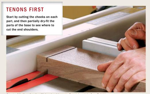
**Start with the cheeks.** Make shoulder cuts first (above), before finishing the tenons on a tenoning jig (below). This sequence allows the waste piece to fall away safely.
