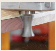
Take it in two passes. After cutting away most of the waste with a jigsaw, make a first pass to remove some of the remaining waste (above), and then reposition the template for a last pass and a smooth final surface (left).
