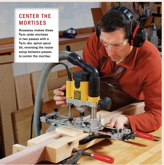
**Solid setup.** Rousseau places the workpiece upside down on the bench and clamps two beams alongside it, flush with the top edge. These provide extra support for a router, which is equipped with two edge guides that hug the beams. Both guides are factory-made, but Rousseau bought longer steel rods to accommodate the beams.
