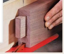
**Center the grooves.** Use a test piece and dial calipers to center the grooves before working on the real workpieces.
