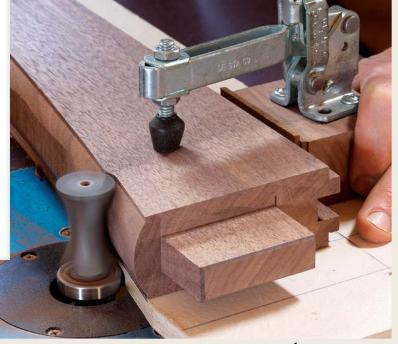
**Rout in stages.** This is a deep cut, so after roughing away the waste, Rousseau inserts ½-in. spacers for a first pass on the router table, and then another set to create the full ¼-in.-wide profile.
