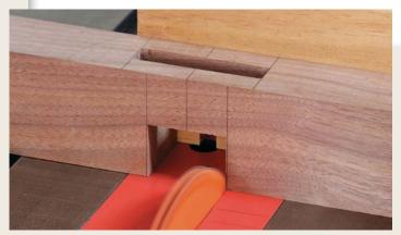
**Nibble to the line.** Using a dado set and an accurate crosscut fence on the tablesaw, sneak up to the pencil line without quite touching it.
