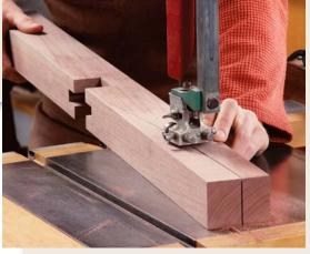
Bandsaw to the line. After laying out the tapers, long curves and rounded tips, bandsaw close to the line. Rousseau smooths the parts with hand tools.
