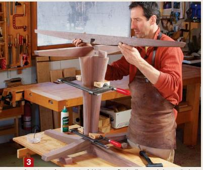
**Last two column parts.** Add the two final splines, and glue on the last two column parts, using curved cauls again. Dry-fit the last foot and arm to be sure to be sure all of the tenons line up with their mortises.
