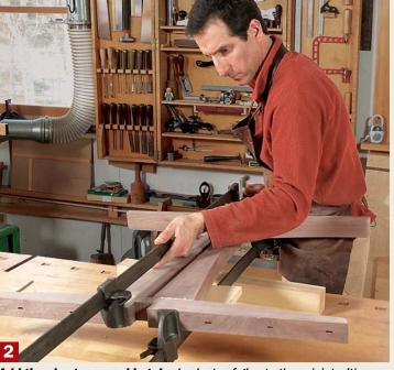
Add the short arm and leg. Apply plenty of glue to these joints. It's better to deal with squeeze-out than to have a glue-starved joint.
