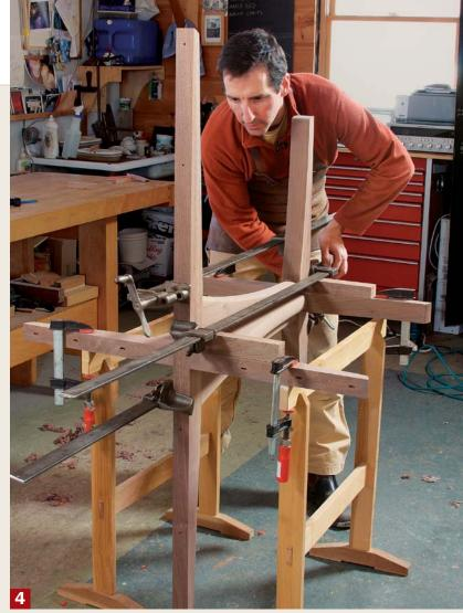
The last arm and foot. To pull the half-laps all the way home, you'll probably need to use bar clamps and a mallet. Rousseau uses epoxy here to buy some extra time.
