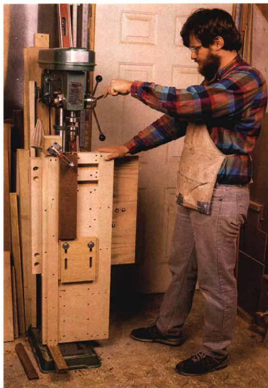
Boring the ends of long workpieces used to present problems for the author, Jeff Greef, until he devised this end-boring jig for his drill press. A pair of platens mounted to the press's table allows adjustments in and out and left and right.
