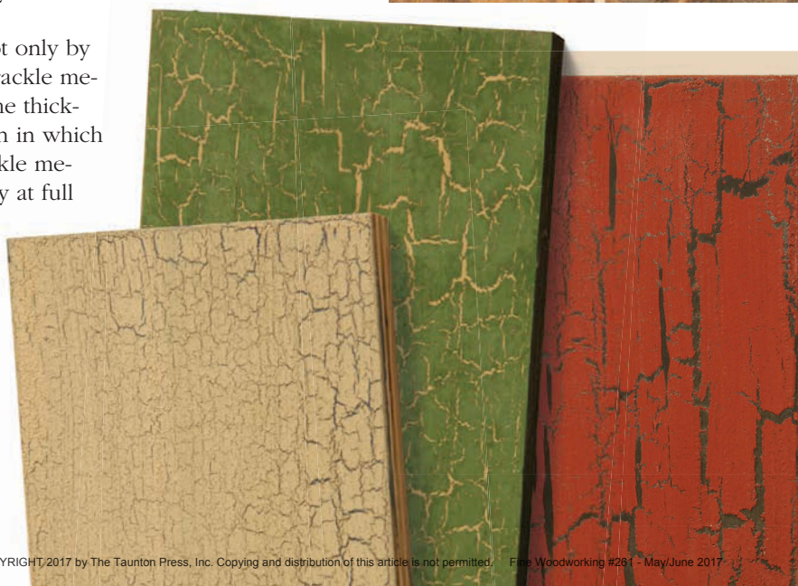
Bold or fine. Use contrasting colors of milk paint for the undercoat and topcoat to emphasize the crackle. Hiller applies the glue coat full strength for a coarse crackle pattern, and thins the glue for a fine crackle.
