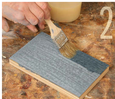
2 Glue coat When the undercoat has dried, brush on a layer of hide glue, the crackle medium.
