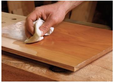
**Re-oil.** With the underlying wood repaired and re-smoothed, apply thin coats of oil to the affected area.
