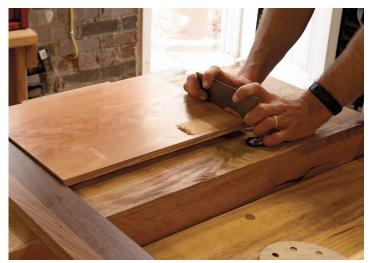
**Deep scratches, gouges, and dents require scraping.** More severe damage requires more work, but it's always simply a matter of returning to the prior luster.
