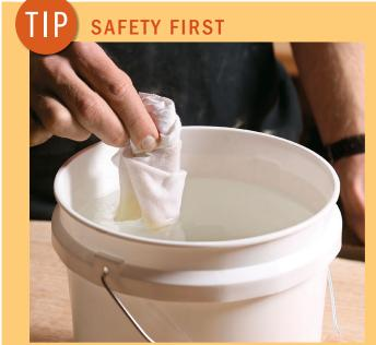
Oily rags present a fire hazard. You should always read and follow the product's safety warnings and instructions for disposal. Generally, Godet soaks the used rags in a bucket of water, which he keeps handy so he can drop in the rag as each coat is done. When he's finished, the used rags go in a plastic bag that he then fills with water, ties up, and puts in the garbage can outside. A sealable jar or other container filled with water also works.
