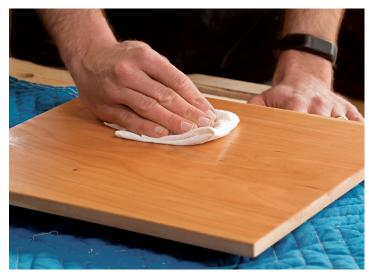
**Wipe and buff.** After the first coat, wait about 30 to 60 minutes before rubbing out the piece with a larger rag. Then, let the piece sit for about 12 to 24 hours, rub it out again with a fresh rag, and apply the next coat. Godet normally applies two to four coats.
