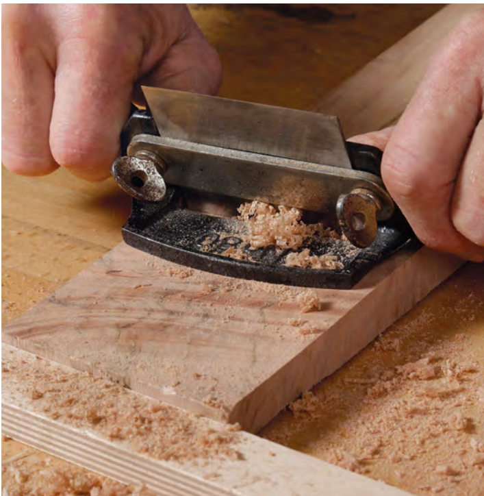
Cabinet scraper. This tool is essentially a scraper held in a spokeshave-like body. Its sole helps it keep surfaces flat, and its handles let you exert more force than with a card scraper.
