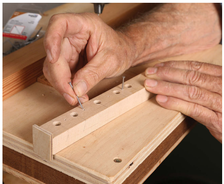
Nails hold the jig in place. You'll affix the jig to the work with two small wire nails or brads. With the jig at the drill press, drill clearance holes for the nails sized to create a little friction, but allow no play.
