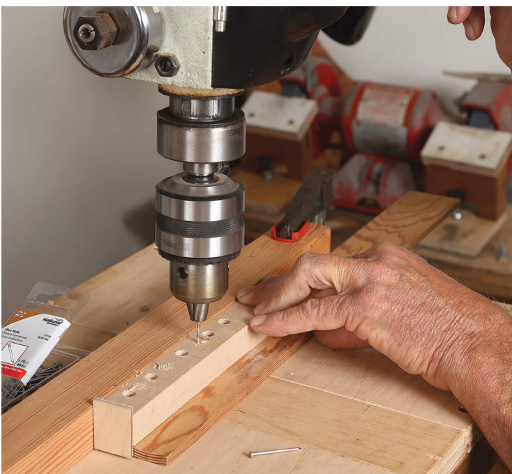
Nails hold the jig in place. You'll affix the jig to the work with two small wire nails or brads. With the jig at the drill press, drill clearance holes for the nails sized to create a little friction, but allow no play.
