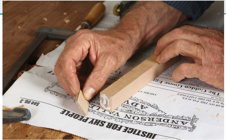
Attach the heel. The jig can be made of any hardwood. Add a \frac{1}{8} -in. to \frac{1}{4} -in. plywood heel to the end of the jig. This will act as a hook to align the jig on the workpiece from the back. Welter chamfers the end of the jig before attaching the heel. This will help keep crumbs from catching in the corner and causing misalignment.
