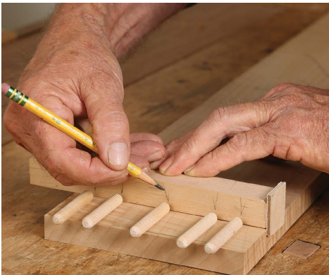
Figure out the spacing. Hook the jig on the workpiece, spread out the dowels, and mark their placement on the jig. Keep the spacing closer at the outside edges, about \frac{1}{2} in. Spread the spacing out to 1 or 1\frac{1}{4} in. toward the center. Drill the holes through the jig on the drill press, positioning them so they'll be centered on the thickness of the workpiece. Then chamfer their edges slightly.
