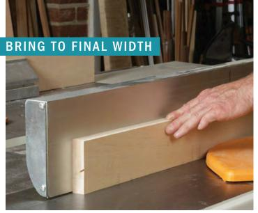
Square an edge to a face. After the rough rip, the board is likely to have crook. If it does, place the concave edge against the table for better stability. This jointed edge will go against your bandsaw fence when ripping.
