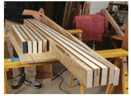
edge will need cleanup and refining. So I rip my finished parts 1/16 in. to 1/8 in. wider than final width, again depending on the part's length. If I'm ripping thinner strips from a wider board, I rejoint a reference edge between passes. The result is multiple pieces of the same width, with one edge jointed and the other edge bandsawn.
