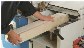
Plane parts to final width. To stabilize narrow parts of the same width, hold them together so they act like a single block of wood. Hold them tightly as they come out the outfeed side, too.
