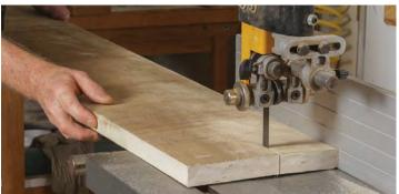
Let the boards acclimate. The rough rips release stress in the wood, causing workpieces to move. To let them work out this movement, O'Malley lays the parts on edge with space between them. He comes back the next day to continue milling.
