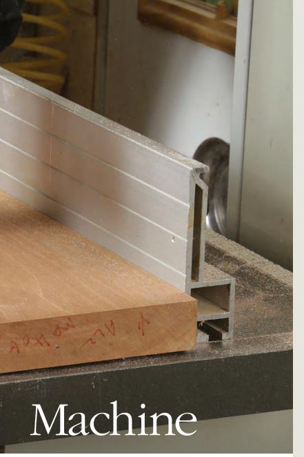
The longer the part, the more extra width I leave in case the part develops crook—a curve along the edge—which is common. There's no need to joint between rips at this stage.
