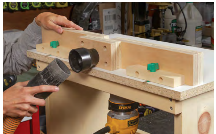
Don't skip the dust collection. The dust port is an easy addition that will keep particulate out of your lungs, eyes, and shop.
