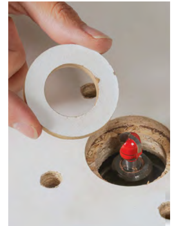
Pick the right insert. The insert closes up the space around the bit, increasing the table's bearing surface and, more importantly, your safety, since stock could tip into this otherwise large opening.
