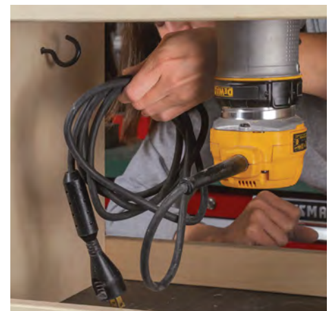
Add a hook for cable management. This keeps the power cord tidy and out of the way when you store your router in the table.
