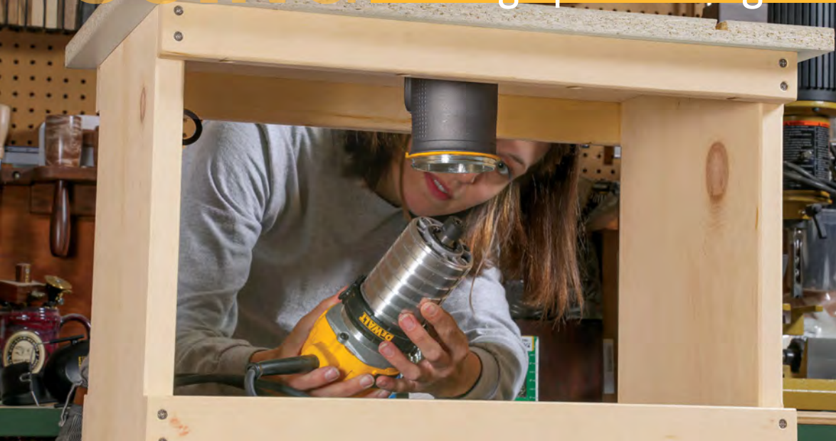
All router adjustments are done under the table. Changing bits requires removing the motor from the base, which stays fixed to the table. Changing the bit height is done via the router's onboard height adjustment.
