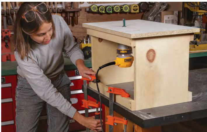
Clamp the table to your bench. Clamps keep the table from scooting around while you're routing. The open base with lower stretchers on the front and back allows for options when securing the table.
