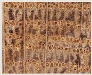
White oak has tyloses. In white oak, the large, earlywood pores are filled with a shimmery material called tyloses, which makes the wood more waterproof and weather-resistant than red oak. And white oak's latewood pores, barely visible at 10x magnification, are much smaller than those in red oak.
