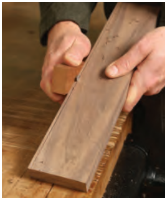
The first half. Take care to keep the fence (i.e., block of wood) tight against your workpiece, and then push and/or pull the tool to scratch a little bead. You may have to play with your angle of attack to engage the screw slot so it's making shavings. This will leave you with the inner half of a bead. Using the same flat block, you can also work a bead along curved edges that aren't too tight, like on the stiles of the chair on the facing page.
