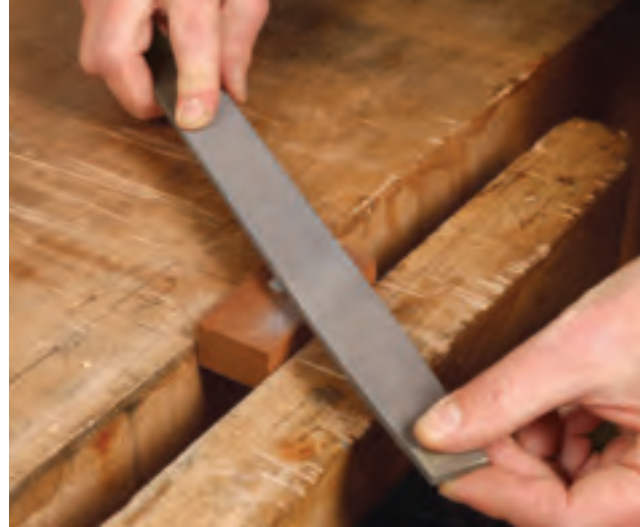
Make the tool. Drill a hole in the middle of a small block of wood, and then use a mill file to flatten the head of the screw and create a sharp edge at either end of the slot.
