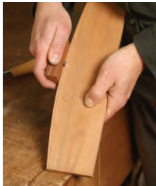
The first half. Take care to keep the fence (i.e., block of wood) tight against your workpiece, and then push and/or pull the tool to scratch a little bead. You may have to play with your angle of attack to engage the screw slot so it's making shavings. This will leave you with the inner half of a bead. Using the same flat block, you can also work a bead along curved edges that aren't too tight, like on the stiles of the chair on the facing page.
