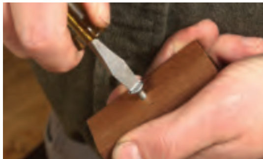
Make the tool. Drill a hole in the middle of a small block of wood, and then use a mill file to flatten the head of the screw and create a sharp edge at either end of the slot.
