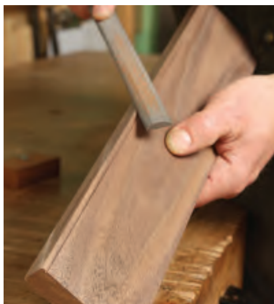
The first half. Take care to keep the fence (i.e., block of wood) tight against your workpiece, and then push and/or pull the tool to scratch a little bead. You may have to play with your angle of attack to engage the screw slot so it's making shavings. This will leave you with the inner half of a bead. Using the same flat block, you can also work a bead along curved edges that aren't too tight, like on the stiles of the chair on the facing page.
