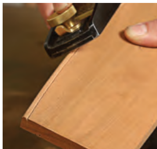
The second half. To get to a finished, full bead, you can easily round over the outer half with a file or a block plane.
