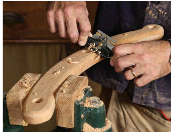
Refine the arms. The arms will receive a lot of attention from the sitter, so use a spokeshave to shape and soften the arms, particularly where the user's hand might wrap around the front or where an elbow might rest.
