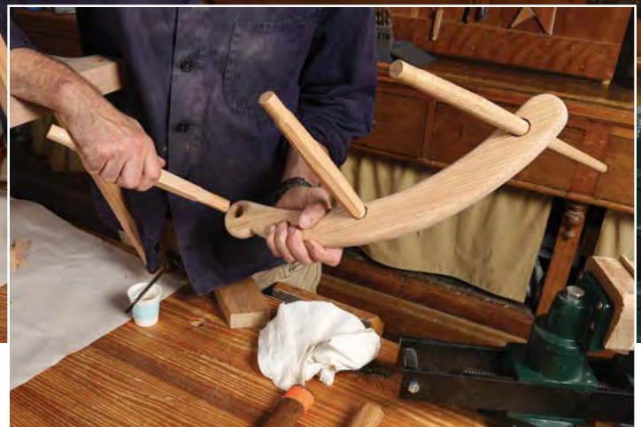
One arm, three sticks. Each arm gets two short sticks and one long back stick. The back stick goes from the seat through the arm to the backrest. First, glue the short sticks to the arm with the back stick in place. Then glue that assembly into the seat. Do the same with the second arm assembly.
