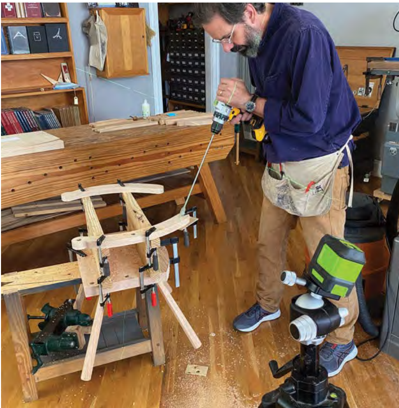
Arm-drilling jig helps with locating arms to seat. A simple jig holds the seat assembly to the armrests while you drill the mortises through the armrest into the seat. A laser level helps keep the hand drill at the right angle.
