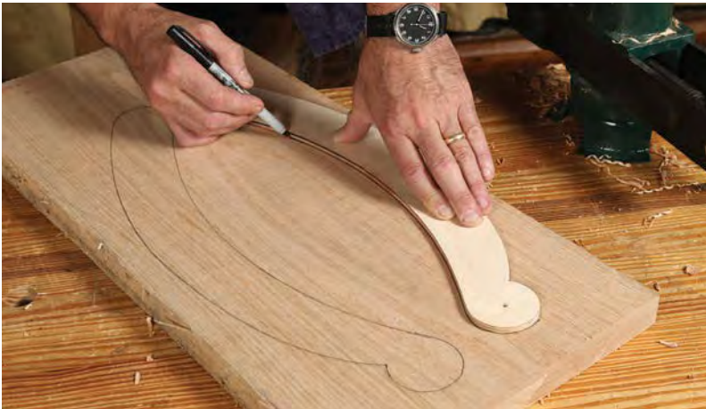
Armrests add curves to the mix. Trace the shape of the armrests, ideally onto one wide piece of stock. Cut out the shape on the bandsaw.
