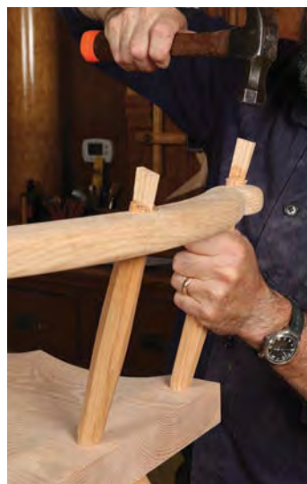
Wedge work. Kerf the tenons of the short sticks and glue in wedges. When the glue dries, cut the tenons flush to the arm.
