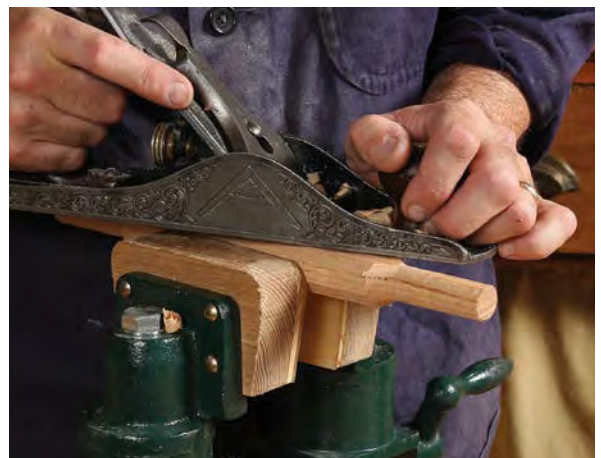
Stick work. Schwarz mills the stock, cuts the octagons, uses a tenon cutter to cut the tenons, and then shapes the sticks with a hand plane.
