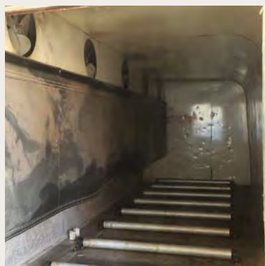
It's windy inside. In conventional kilns like this one, fans circulate the heated air, driving it around and through the lumber stack.
