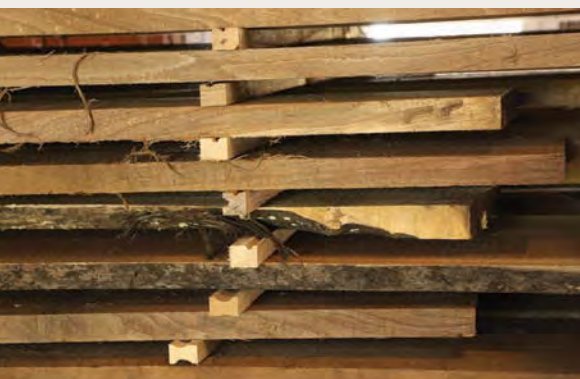
Stacked right. Conventional kilns, which rely on surface evaporation to extract moisture from wood, require green planks to be stacked on stickers, creating airways between layers of lumber. Schucker mills specially shaped stickers that reduce the chance of sticker stain.
