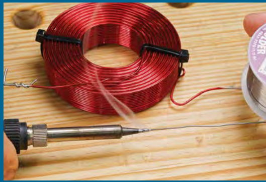
Step 1: Tin the iron. Melting a little bit of solder on the tip of the iron helps the iron transfer heat to whatever you touch.
