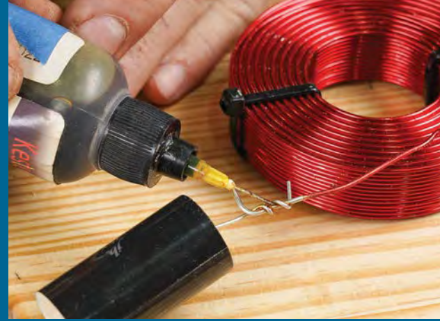
Step 2: Add some flux. For wire-to-wire connections like these, it helps to add a small amount of liquid flux to the joint.
