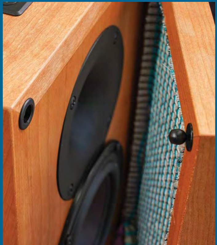
Shape the parts. Bevel the edges of the parts, rabbet them for the grill fabric, and bandsaw curves along their inside edges.
