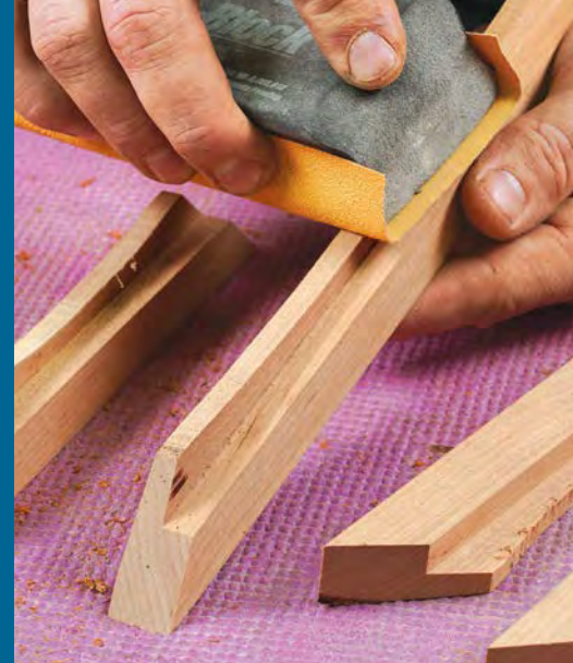
Smooth the sawcuts. After mitering the ends of the parts, plane and/or sand them smooth.
