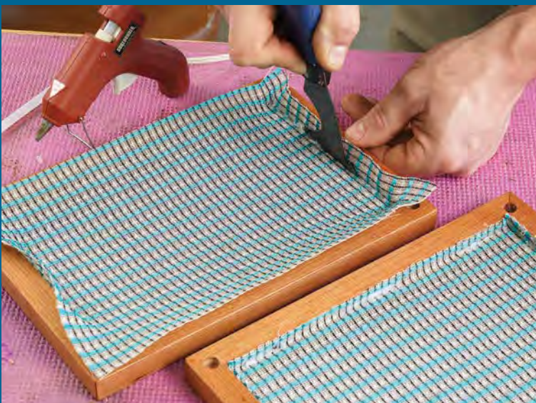
Add the fabric and install the grill guides. To anchor the grill fabric in the rabbets, squirt a bead of hot-melt glue into the corner, and push the fabric into the rabbet using a paint scraper, holding it there while the glue cools. Start at the centers of the short sides and work toward the corners, applying glue by folding back the fabric (above). Then do the same along the long edges. Next, install the grill guides (right). These inexpensive but handy guides (from Parts Express) include a little knob and a small receiver that click together, making it easy to attach and detach the grills.
