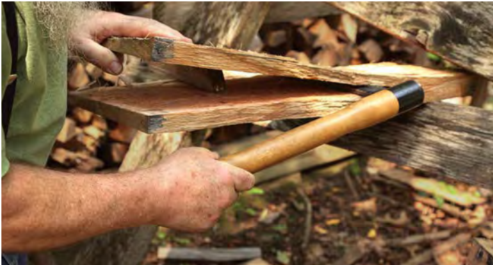
Excess thickness. Most splits are tapered in thickness. You can rive off some of the excess with the froe. Jam the stock into the bars of a riving brake and work the froe forward as you push down on the handle to open the split. Use a piece of scrap to keep the split open behind the froe, making it easier to advance.
