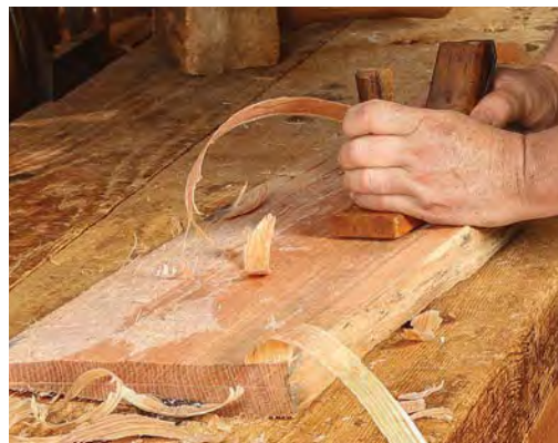
A scrub plane follows the froe and hatchet. It starts to bring the riven, hewn blank toward something flat and smooth. Jam the workpiece against the iron-toothed bench hook or planing stop.
