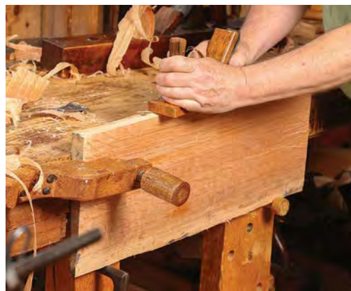
Edge jointing. Here the board is pinched against the edge of the bench in a wooden screw/crochet. Its front end sits on a holdfast, its back end on a peg in a sliding deadman.
