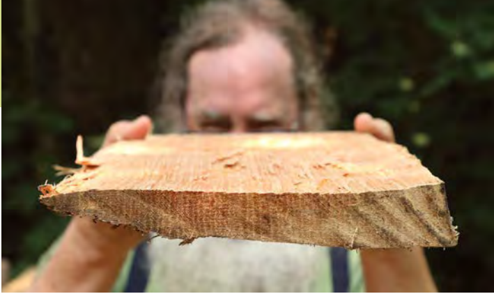
The perfect log. When you find perfect logs, which are rare, they are the greatest thing. This radial plane is flat along its length and width.
