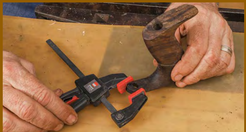
Light clamping. Moderate pressure from a light-duty quick-release clamp is adequate to close a repair when using epoxy.
