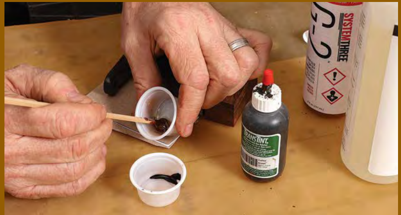
Mix and color the adhesive. For almost all repairs of the furniture on user planes, Addison glues with System Three G2 epoxy, which he mixes and then colors with a tiny dab of TransTint.
