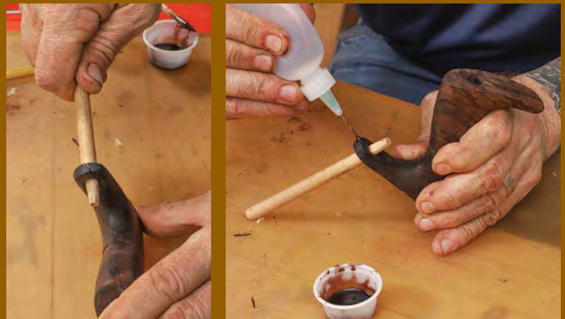
A split in the toe of the tote. To remedy this minor defect, which is common in vintage planes, Addison tapers one end of a dowel and twists it into the screw hole at the toe of the tote. This opens the crack in the toe enough to deliver some epoxy using a syringe bottle.
