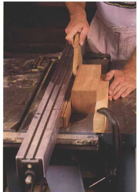
Resawing reconsidered —A chunk of 4x4 screwed to a stick is all that it takes to keep the stock vertical and the blade safely hidden while resawing. If you resaw often, you can screw the guard block directly to a dedicated throat plate.
