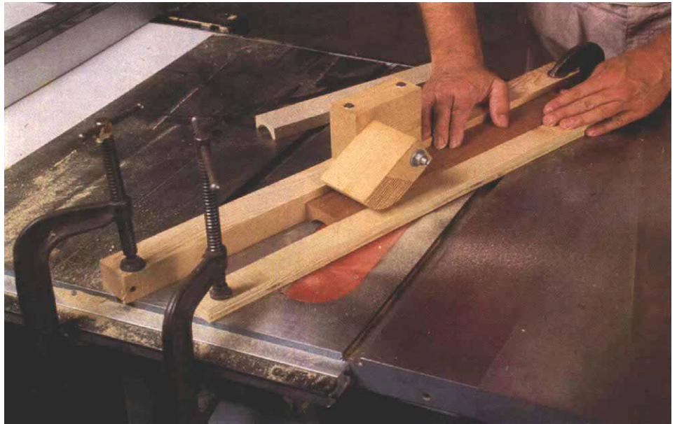
Wide featherboards are excellent for coving —They exert downward pressure over the cutting area while keeping hands from coming near the blade.
