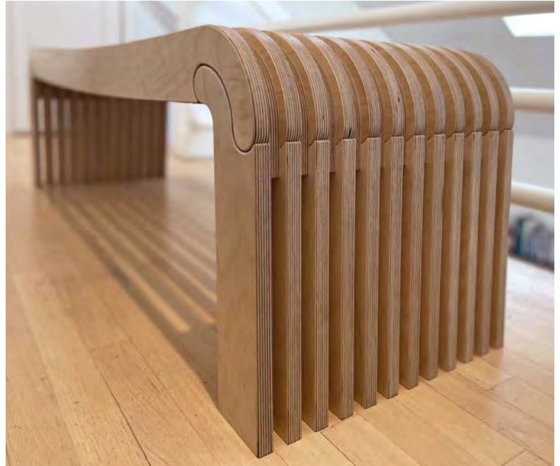
Overlapping legs and seat. The Olap Bench consists of a seating surface with ends that overlap its legs. The legs and the seat slats terminate in nesting half rounds, forming an S-shaped jointline. Furbershaw likes to take advantage of the capabilities of CNC machining to create visually interesting joints like this.
