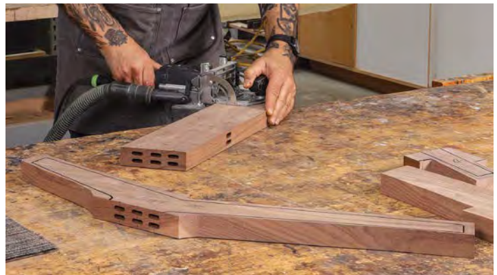
Portable mortising. McGlasson used to use a stationary mortiser when joining the side parts, but now he finds the Domino far more convenient.
