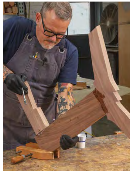
Slow assembly. Epoxy's long open time permits you to assemble the whole side (except for the armrest, which is added later) in one go. A hand-screw clamp keeps the parts upright as you seat the front leg.
