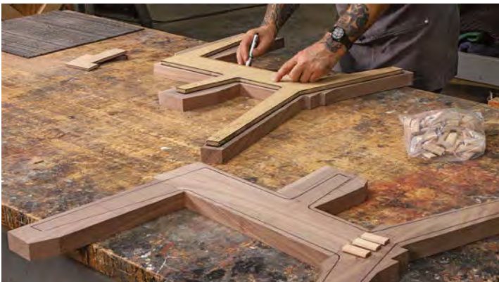
Place and trace. With all the side parts sawn out and their mating surfaces flattened, put them in position and trace the finished template onto them. Also, mark the joints for Dominos.
