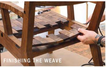
**Tilework, part 2.** With the front half of the seat's tilework woven, start weaving again with a fresh piece of rope from the back. For the final pass of the rope to connect the front and back halves of the seat's tile field, tip the tiles up and down as needed, pull the rope tight and thread it back through the extra hole in the side, and secure the end to the second cleat.
