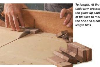
table saw, crosscut the glued-up pairs of full tiles to make the one-and-a-halflength tiles.
