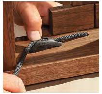
Cleat tightening. With the rope pulled through to the inside, cinch it tight in the rope cleat. Then cut off the excess rope and torch the end.
