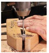
**Custom clamping.** To hold a bead securely while drilling through it, you can customize a hand-screw clamp: use a Forstner bit to cut a shallow hole in the jaws to fit the bead.
