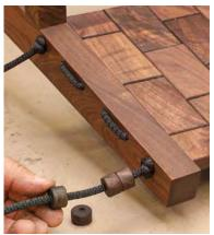
**Thread the beads.** Lace on a few beads to decorate the top knot of the chair's back. Then tie off the rope, cut it, and torch it.
