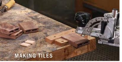
**Special tiles get mortised.** One-and-a-half-length tiles begin every other row in the tile field to create the running-bond pattern. To make them, join two full tiles with Domino slip tenons. Three scraps screwed to the work surface keep the tile stationary while it's being mortised.
