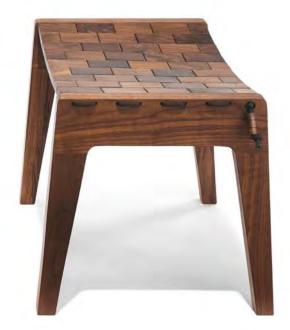
he solid wood tiles on my chairs are strung on high-grade polyester rope pulled taut between the sides of the chair. I arrange the tiles in a running-bond pattern (borrowed from brickwork), which is visually attractive but also links the tiles together in an interlocking web.
