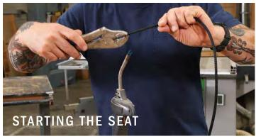
**Rigidified rope.** McGlasson likes the rope to fit tight in the tile holes. To make threading the rope easier, create a firm, thin section at the leading end of the rope by torching the first few inches, pulling and twisting the rope slightly as you do so.
