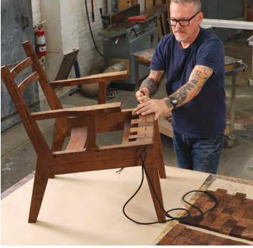
**Weaving a pleasing pattern.** Before you begin the weaving, lay out all the tiles in an appealing arrangement, bevel the outside edges of the side tiles, and sand and oil the tiles one by one, carefully replacing them in the original pattern.
