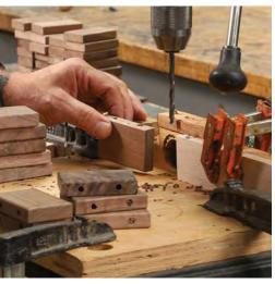
**Drilling station.** With a brad point bit at the drill press. drill holes through all the tiles. To avoid chipout, drill halfway through. then flip the tile to finish the hole from the opposite edge. A vacuum port in McGlasson's shopmade fence keeps the tile sucked tight during drilling, then evacuates chips when the tile is pulled away.
