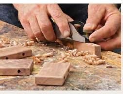
Angled edges. Make the initial bevel cut at the bandsaw with the table tilted, then smooth the sawn surface with a block plane.
