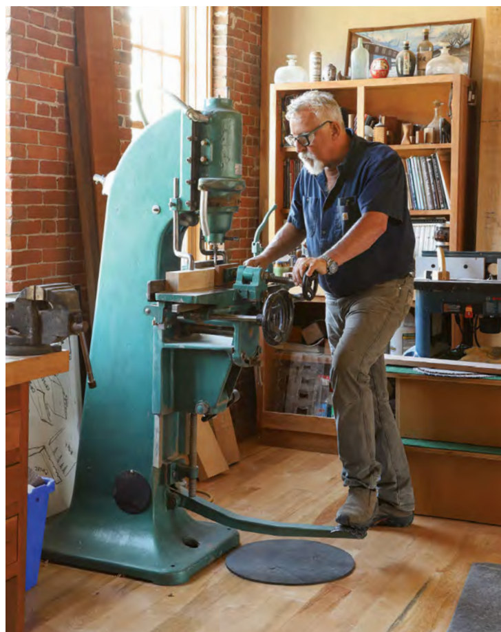
Lots of leverage. Most of Moriarty's chair parts get mortised on this 1947 Oliver mortiser, which he fully restored.
