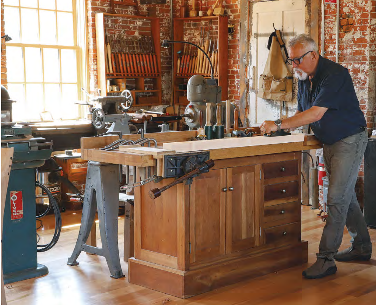
It's not all iron. Moriarty built his Shaker-style workbench with a maple top and ample storage below, and outfitted it with an Emmert patternmaker's vise.
