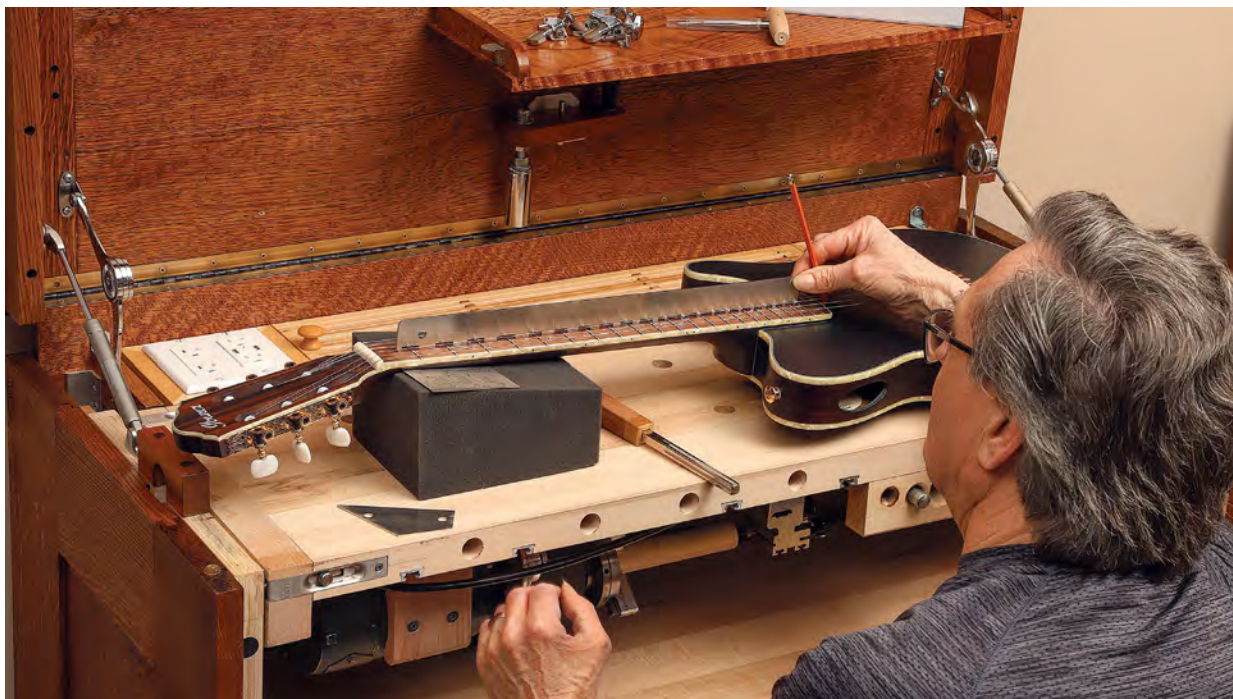
Small bench for big passions. This cabinet is intended as a richly featured workspace for pursuing crafts and hobbies of relatively limited scope. In addition to a workbench, it offers shelving, ample drawer storage, a micro lathe, a retractable desk, air filtration, and power outlets. An avid guitarist, Baker finds it useful when adjusting the neck of a guitar.
