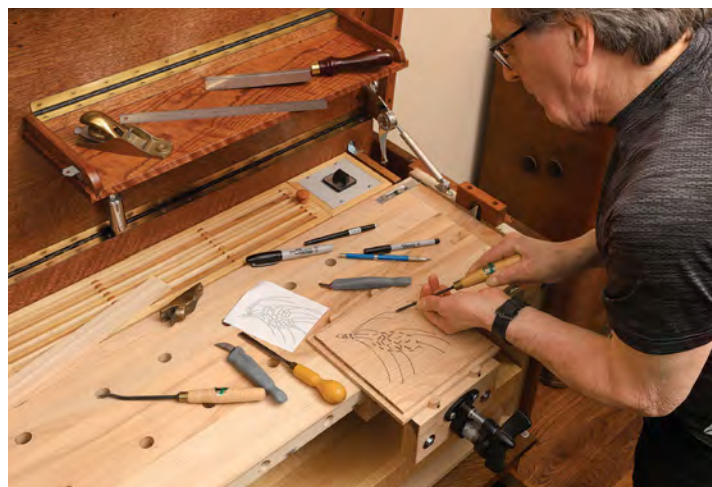
Quick, add a vise. A Lee Valley pipe vise that Baker modified lives in one of the cabinet's drawers until it's needed, when it slides in and goes to work in a blink. Chip carving nicely suits the scale of work accommodated by the cabinet.
