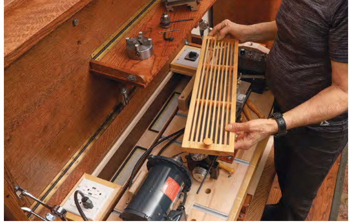
Air filters. A grille behind the bench slab covers a pair of exhaust fans that pull light sawdust into HEPA charcoal filters.
