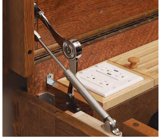
Stay strong. Dual cabinet stays on each end help lift the solid-oak lid and secure it in its open position.
