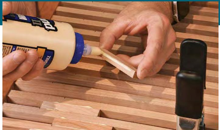
**Gluing tips.** To install a filler block, apply glue lightly to its sides, but not to the spindles. Keep the glue near the back edge of the block and away from its ends, where excess will be hard to remove.
