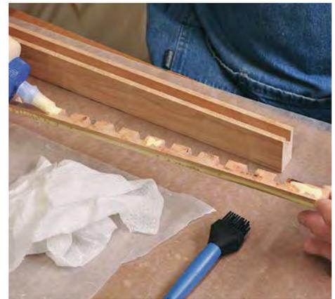
**Where to apply glue.** Place glue on the strips only, applying it along the bottom and sparingly on the sides near the notches, where squeeze-out will be difficult to remove.
