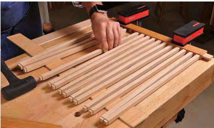
**How to manage the spindles.** The spindle tenons are inserted dry. Clamp one rail to the bench and fit its spindles. Note the spacer strip that keeps the spindles level, making assembly easier. Then, starting at one end of the opposite rail, insert the rest of the tenons.
