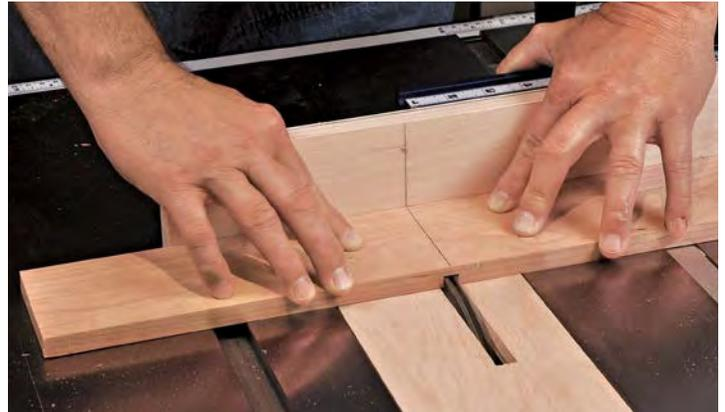
**Center the first dado.** Mark the center of the strip, set up a dado set to cut a dado that's  $\frac{3}{8}$  in. wide and  $\frac{9}{32}$  in. tall, and center it on the mark.
