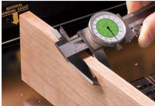
**Plane the strip board.** The strips are cut from a wider board. Plane that board until its edge fits snugly in the rail grooves.
