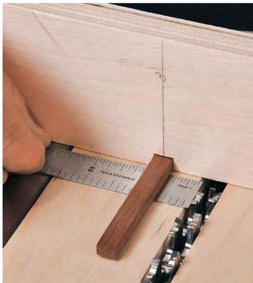
**Set the spacing.** Slide the fence along your miter gauge until the key is exactly  $\frac{5}{8}$  in. away from the outer blade. Reattach the fence in that position.
