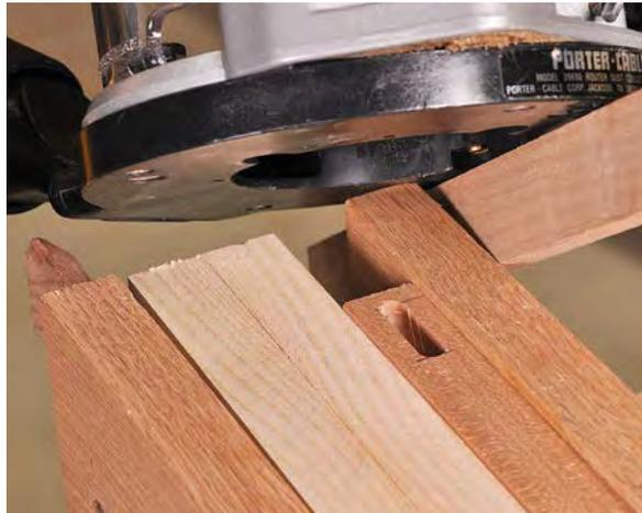
**Clean results.** Trust your eyes to stop the mortises at the pencil marks. The mortise length is not critical as long as it reaches the marks.
