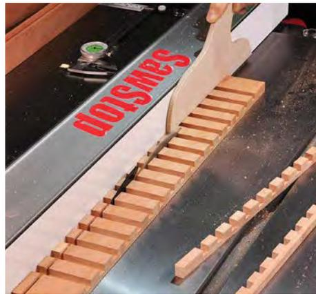
**Rip the strips.** Cut the notched board into strips that fit snugly into the rail grooves.
