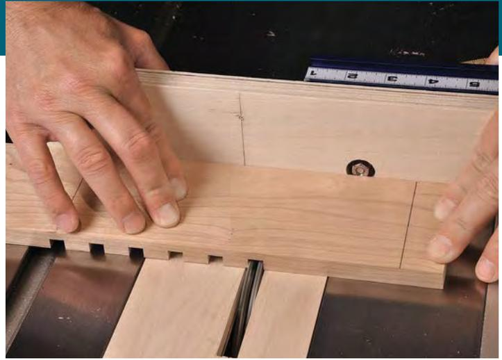
**Cut half of the notches.** Use the jig to cut a row of notches in your real strip stock, starting at the center and moving toward one end, stopping short of the tenon area (marked).
