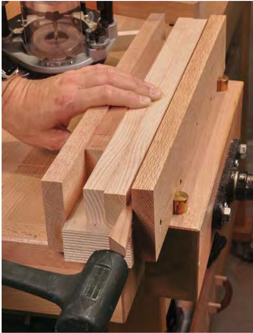
**Dial in the edge guide.** Lay out a mortise on a test piece, and adjust the router's edge guide to align the bit with the layout.
