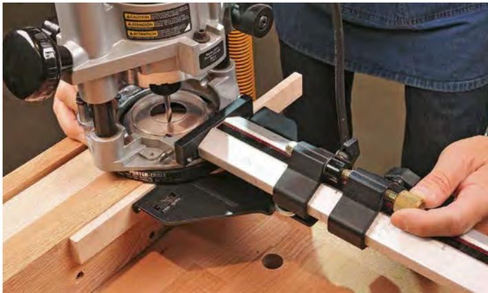
**Make a few test plunges before mortising the stiles.** Measure with dial calipers to make sure the mortises will be centered (right). Mark the beginning and end of each mortise, and cut each mortise in a series of passes, using the depth stops on your plunge router (far right).
