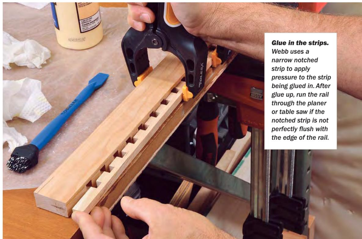
**Glue in the strips.** Webb uses a narrow notched strip to apply pressure to the strip being glued in. After glue up, run the rail through the planer or table saw if the notched strip is not perfectly flush with the edge of the rail.
