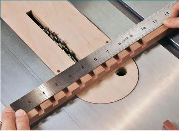
**Cut a test strip.** Use the indexing jig to cut a row of notches in a test strip. Spacing errors are cumulative with this jig, so you'll see them at the end of the row. Adjust the fence position and do another test if necessary.
