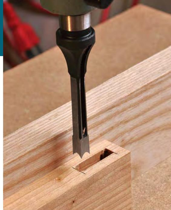
**Square the mortises.** You can do this with a small chisel, or use a mortising bit in your drill press, as shown, with the drill bit removed.
