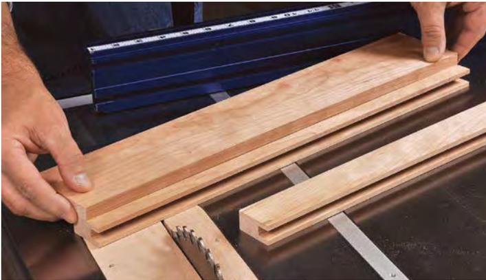
**Cut it to length.** Cut the strip board to the same length as the rails. Then add a plywood auxiliary fence to your miter gauge (see photo at right).
