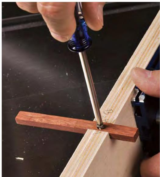
**Add a key to the auxiliary fence.** Cut a  $\frac{1}{4}$ -in.-thick by  $\frac{3}{8}$ -in.-wide slot in the fence, and screw a  $\frac{3}{8}$ -in.-wide hardwood key into it as shown.
