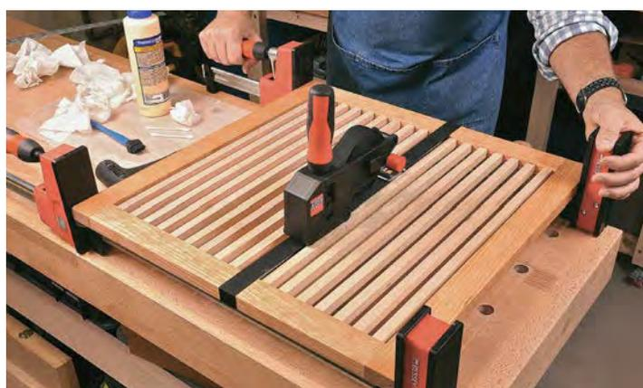
**Add the stiles.** Hold the rails and spindles together with a strap clamp, apply glue to the mortises and tenons in the frame, and clamp the stiles in place. Make sure the assembly is square.
