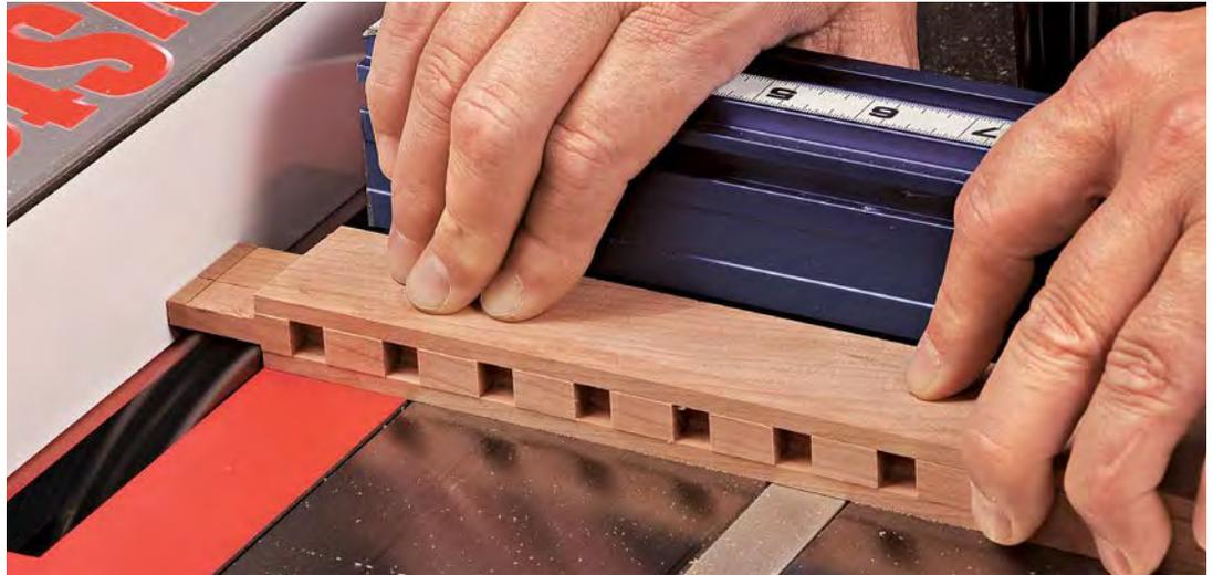
**Tenon the rails.** Load a wide dado set in your table saw, support the workpiece with the miter gauge, and use the rip fence as a stop.
