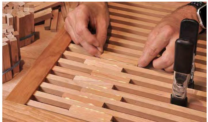
**Blocks go in from the back.** Push them in until they are flush with the back of the spindles and aligned with the pencil marks on the spindles that denote their locations. Note how squeeze-out is pushed to the back of the assembly, where it is easy to remove.
