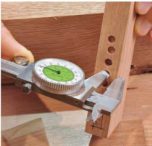
error will accumulate along the row of notches—so check it by cutting a series of notches in a scrap board. If there is an error, adjust the location of the indexing jig slightly and cut more test notches. When you are happy with the spacing, place that first dado you cut onto the indexing key and cut the next notch and then the next, continuing until you reach the end of the row, which should stop right before the mark for your tenon shoulder.
