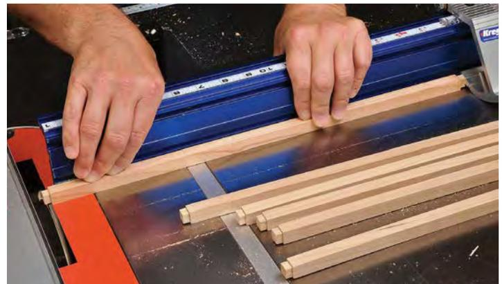
**Tenon the spindles.** First, dry-fit the frames to determine the spindle length and the distance between their tenon shoulders. Then cut them to length. When tenoning them, set a stop at the far end of your miter gauge.
