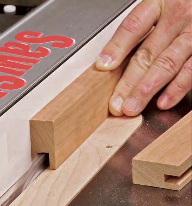
**Slot the rails.** Webb used a  $\frac{1}{4}$ -in.-wide dado set here, running the workpieces in both directions to create  $\frac{3}{8}$ -in.-wide grooves centered on the rails.
