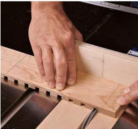
**Cut the other half.** Flip the stock around to cut notches in the opposite half, starting at the center again.
