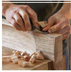
Slice to a shallow curve. Using a drawknife or a hand plane, shape the sides to follow the outer curve you drew out with the drawing bow. The curved surface you create should be plumb for now.
