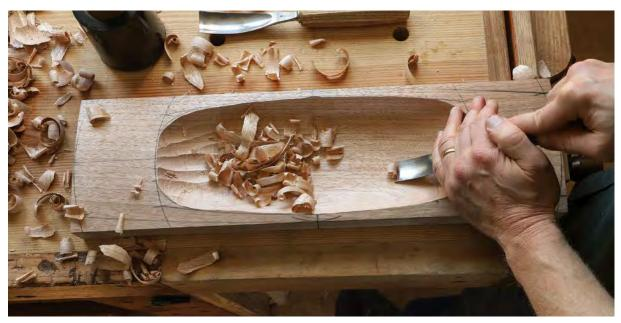
**Finessing the hollow.** When you're happy with the shape you've carved for the hollow, put the mallet aside and refine the surfaces with paring cuts using the flatter #5 gouge. Fisher likes the surface left by the gouge, but for a completely unfaceted surface you could follow up with sandpaper or a gooseneck scraper.
