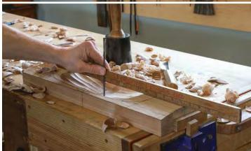
**Depth check.** When you've carved a lateral trench that feels close to full depth, check it with a straightedge and a narrow ruler. You want to leave about <sup>1</sup>/<sub>4</sub> in. of meat below the trench.
