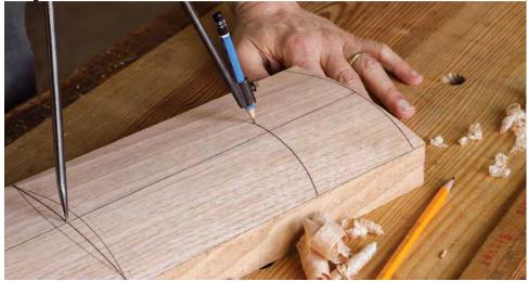
**Scribing from the center.** Draw crossing centerlines on the newly crowned top surface, then strike arcs with a compass placed at the center point and set to a  $10^{\frac{1}{2}}$ -in. radius for the ends of the handles and a 7-in. radius (as shown above) for the ends of the hollow.
