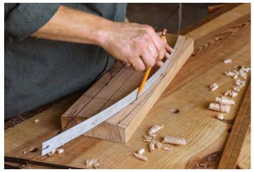
**Drawing bow sets the side curves.** To lay out the sides of the bowl and the hollow, line up a drawing bow with the end and middle tick marks.
