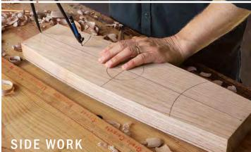
**Layout underneath.** First, with the compass point placed at the intersection of the centerlines, draw a 3-in.-dia. circle to establish the width of the foot. Then, as shown above, draw 4<sup>7</sup>/<sub>8</sub>-in. radius arcs across the blank at both ends to define the end-curves of the foot.
