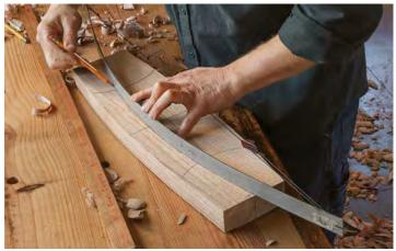
**Arc of the foot.** To define the side of the foot, adjust the drawing bow so it connects the center points at both ends and is just tangent to the center circle.
