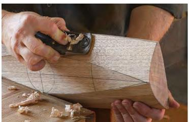
**Now the fun part.** After the careful layout, shaping is a breeze. Rough out the shape with a drawknife, creating a curved surface that connects the almond-shaped layout lines on the bottom and the line along the side just below the lip. After using the drawknife, you can smooth and refine the surface with a block plane or a spokeshave.
