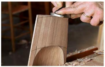
**An arc at the end.** Once the underside of the handle has been roughed out, use a drawknife or hand plane to shape the end to a curve.
