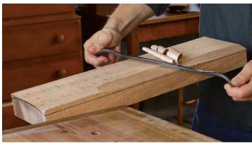
**Rough in the curve.** Using a drawknife—or a hand plane set to take thick shavings if you prefer—crown the top surface of the blank from end to end.
