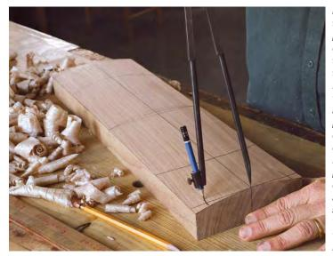
Define the widths. Set the compass at 25/16 in., place its point on the centerline, and strike two short arcs across the handle curve (left). Repeat the process with the compass set at 21/16 in. and its point placed where the end curve of the hollow crosses the centerline. Last, with your compass point at the intersection of the centerlines, draw arcs with the compass set at 3 in. and  $2^{11}/16$  in. These will mark the widest points of the bowl and the hollow.
