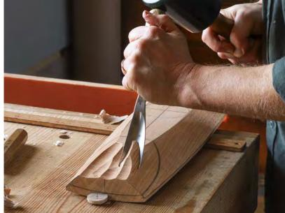
**Hewing out the handle.** Rough out the underside of the handle with the #8 gouge and mallet. Begin with short scoops started not far from the end of the bowl and working backward with longer cuts.
