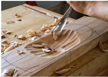
**Retrenchment.** After you've reached the bottom of the original crossgrain trench, carve a deeper one, then continue making longer and deeper parallel cuts with the grain.
