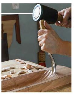
**High up at the ends.** Make the final cuts at the ends of the hollow with the gouge nearly vertical to establish steep walls.
