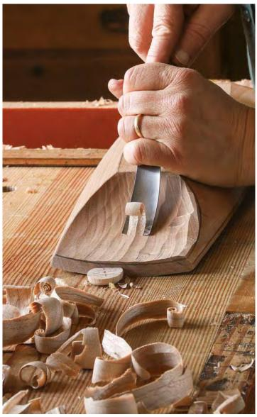
**Finishing up.** Shift to paring strokes at the end to refine the curves and smooth the surface.
