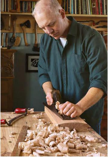
**Complete the crown.** After roughing in the curve, smooth it with a finely set hand plane or spokeshave.
