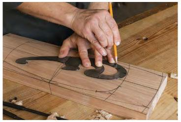
**Curves into the corners.** You can use a French curve to round the corners of the hollow.
