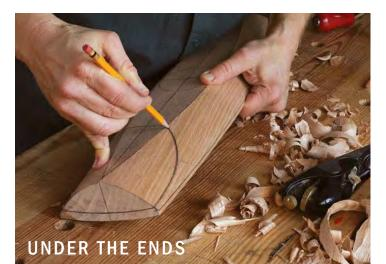
**Handle layout.** With the sides shaped, lay out the handles by first drawing a line on the end grain <sup>3</sup>/<sub>8</sub> in. below the top. Then, beginning at the end of that line, draw a curve that ends at the corner of the foot.
