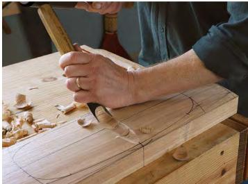
**Trench work.** Begin the excavation of the hollow by carving a lateral trench about <sup>1</sup>/<sub>2</sub> in. deep with a #8 gouge and a mallet.
