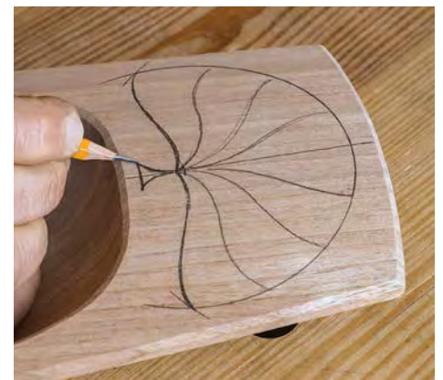
Last layout lines. Working by eye again, draw a series of curving lines to divide each half of the crown into four sections. Then draw the triangular trunk with three slightly curved lines.
