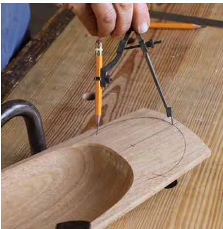
Arc of the foliage. Draw an arc with the compass set to 2\frac{1}{4} in. and its point on the centerline \frac{7}{8} in. from the bowl's hollow. Then, as shown here, draw two tick marks on the arc with the compass set to 3\frac{3}{8} in.
