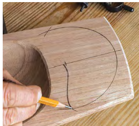
Enclosing the crown. Working by eye, draw an S-curve from the centerline to the tick mark on the outer arc. Make a second S-curve on the other side to complete the bottom edge of the crown.
