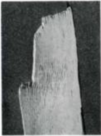
This maple veneer is so loose that the surface is corrugated.
