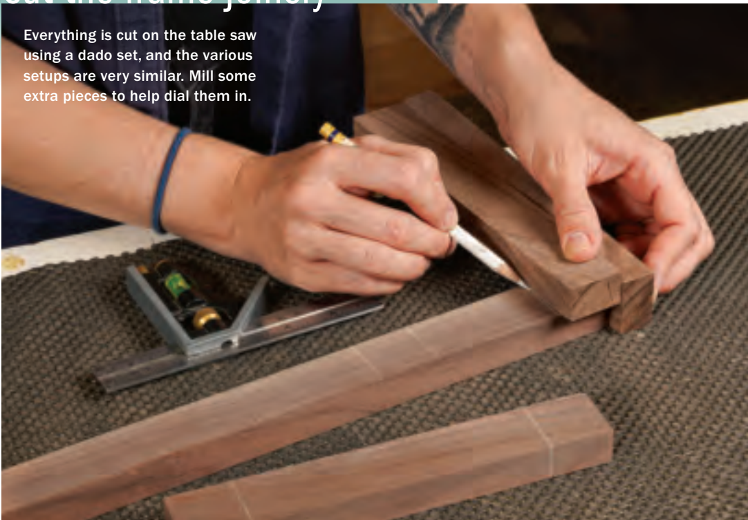
Lay out the lap joints. To ensure a good fit, Amick used mating parts to lay out the large rabbets and notches. A white pencil shows up nicely against the dark walnut.
