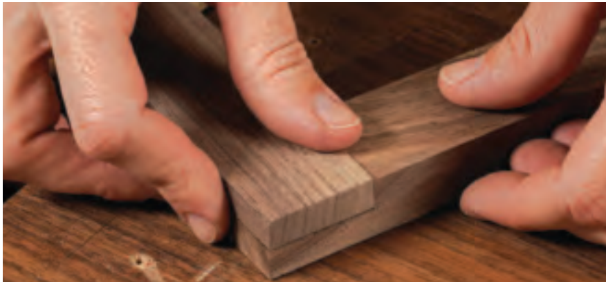
Lay out the lap joints. To ensure a good fit, Amick used mating parts to lay out the large rabbets and notches. A white pencil shows up nicely against the dark walnut.
