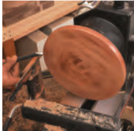
True the perimeter. A \frac{5}{8} -in. swept-back bowl gouge, making passes toward the headstock, quickly trues the perimeter of the blank.
