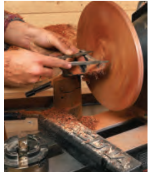
Getting ready for a recess. With both faces flat, adjust a pair of dividers to the diameter of your four-jaw chuck, then transfer that measurement to the blank. You'll turn a recess here to accept the chuck.
