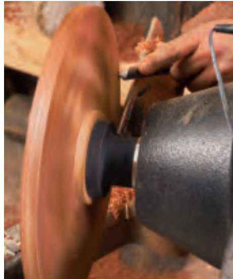
True the inside. Monaco uses a wing of the \frac{5}{8} -in. swept-back bowl gouge to shear scrape the other face of the blank.
