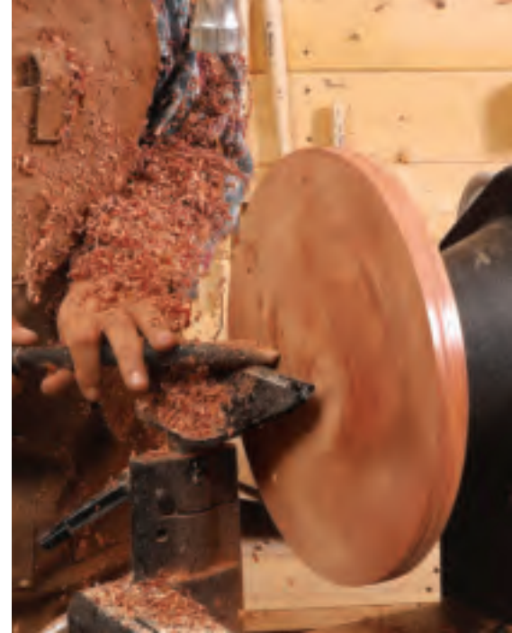
Flatten the bottom face. Again using a \frac{5}{8} -in. swept-back bowl gouge, true the bottom face of the dish blank.
