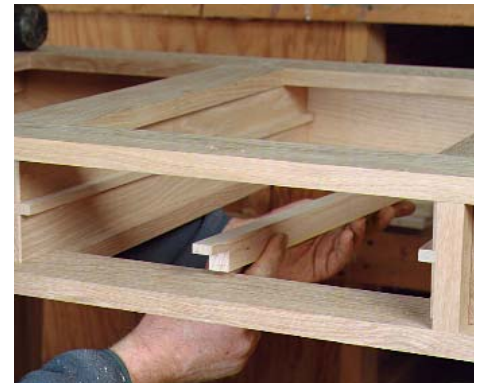
Insert the drawer glides and install the center glide. Glue the drawer glides in place and mount the center glide on the lower drawer frame. The center glide ensures that the drawer tracks correctly.
