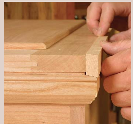
The lid molding masks minor warp or twist in the frame-and-panel. Set the lid on the box and apply the molding so that it rests on the edge of the carcass molding.
