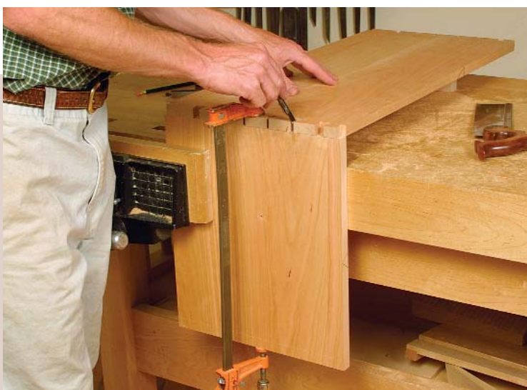
Mark the pins with the tails as your guide. With the tail board clamped firmly in place, trace the tails onto the end grain of the pin board with a marking knife. Deepen the marks with a chisel to provide a kerf for the handsaw.
