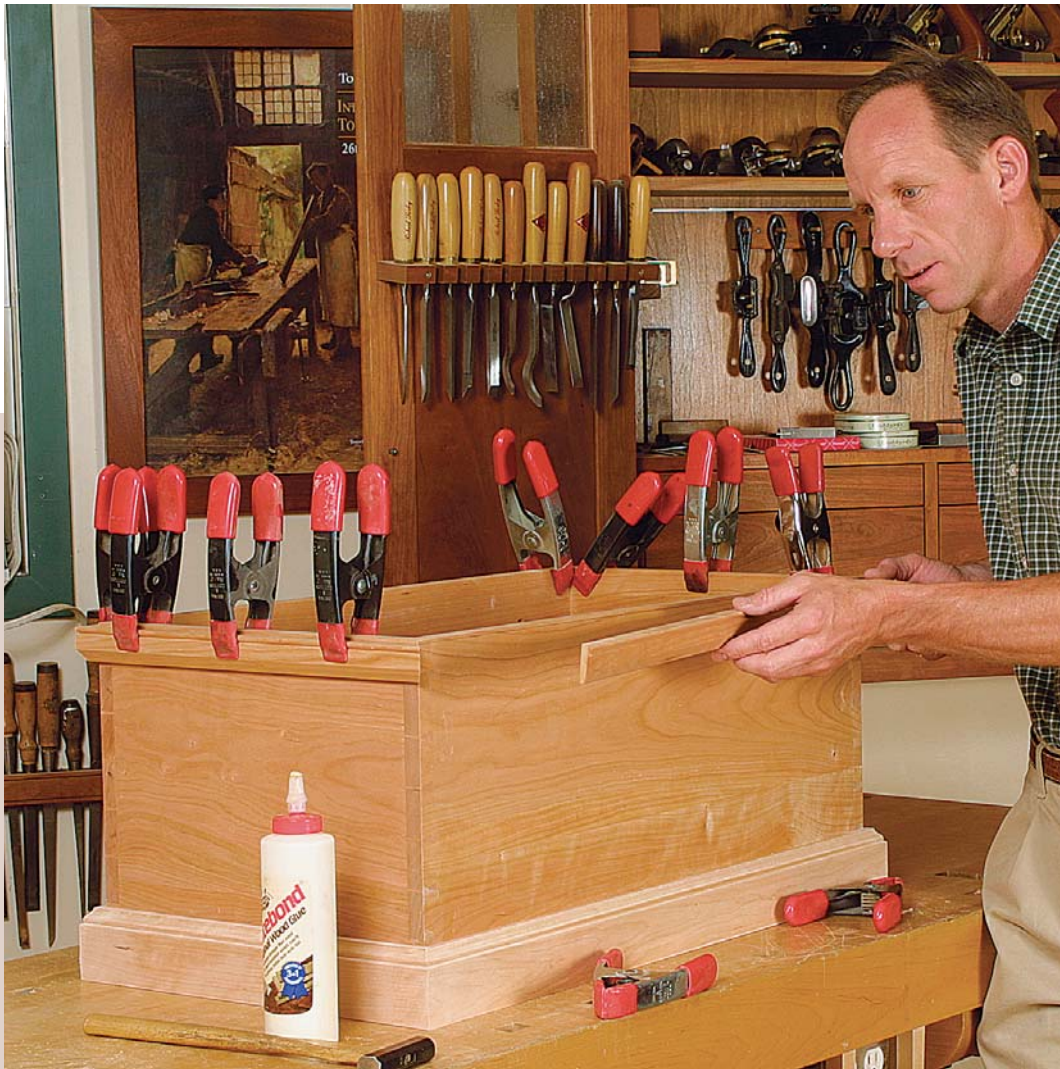
Glue the top molding. Later, after the hardware has been installed, nail the molding with finish nails to add additional holding power.
