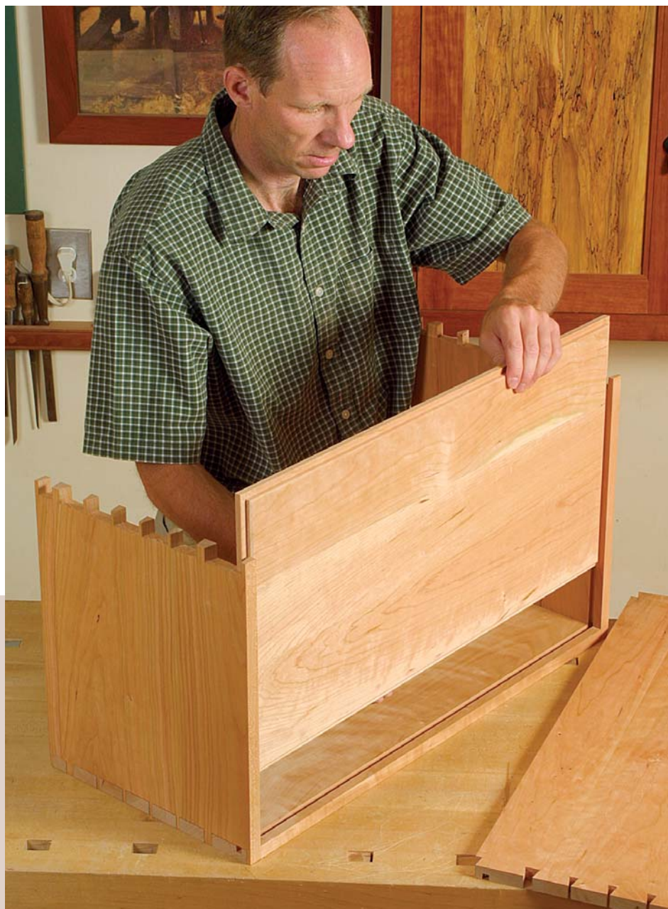
Glue up the carcass. After dry-fitting all of the pieces, coat the dovetail joints with slow-setting wood glue and assemble. The rabbeted bottom panel floats in the grooves plowed into the four sides. No glue is used.
