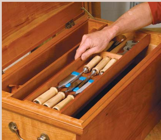
Dovetailed trays hold hand tools. The three trays are sized specifically to hold Gochnour's chisels, planes, saws, and various other hand tools. The sides are dovetailed, and the bottom panels are glued flush to the trays.
